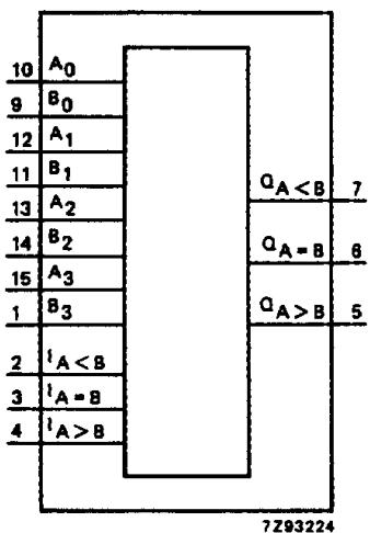
Fig.4 Functional diagram.
