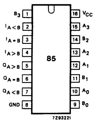
Fig.1 Pin configuration.
