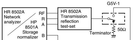
Terminals which were not being measured were terminated with 50Ω.
