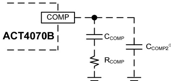
①: C<sub>COMP2</sub> is needed only for high ESR output capacitor
