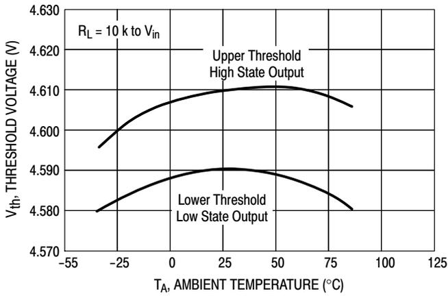
Figure 4. Comparator Threshold Voltage versus Temperature
