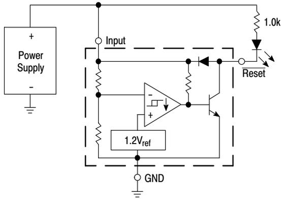
Figure 11. Voltage Monitor
