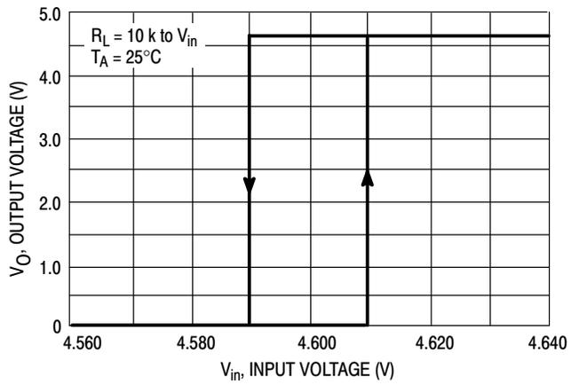
Figure 3. Reset Output Voltage versus Input Voltage
