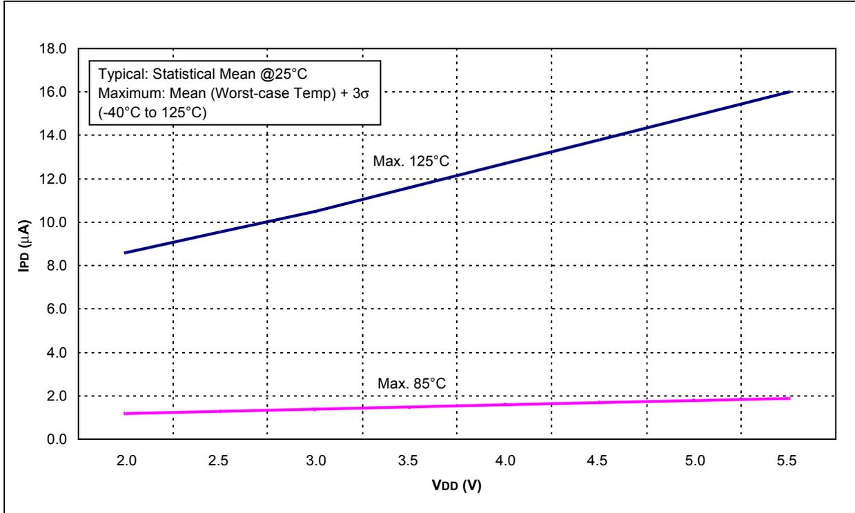
FIGURE 18-15: COMPARATOR IPD vs. VDD (BOTH COMPARATORS ENABLED)
