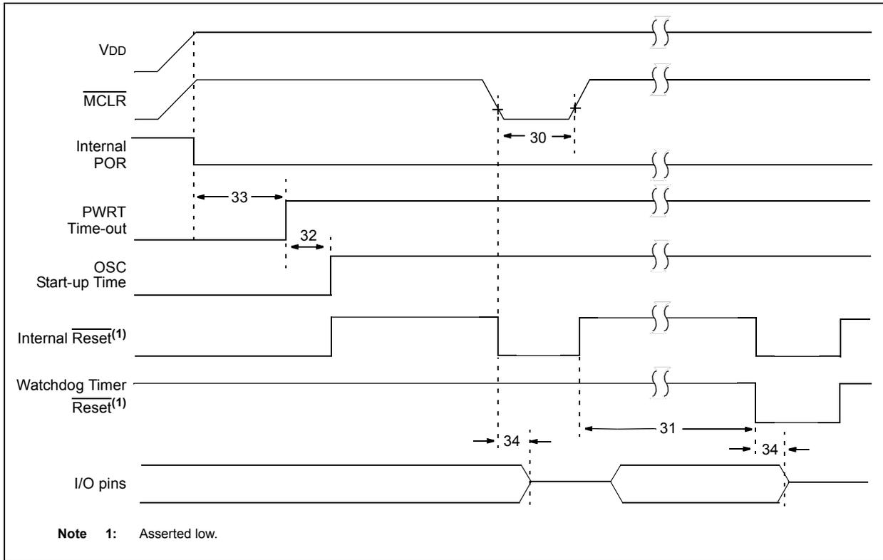
**FIGURE 17-7: BROWN-OUT RESET TIMING AND CHARACTERISTICS**
