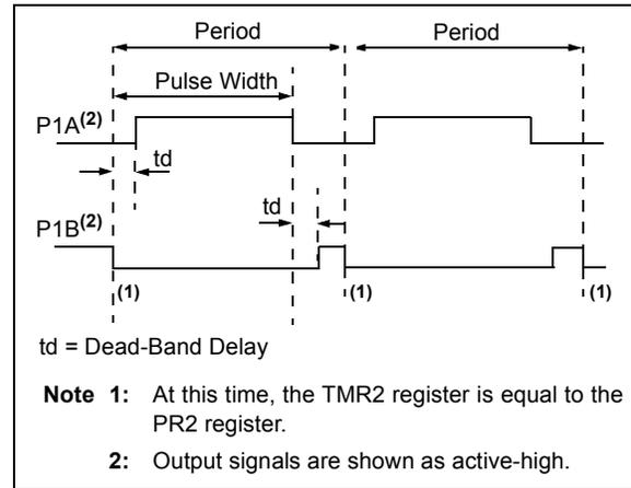
**FIGURE 11-9: EXAMPLE OF HALF-BRIDGE APPLICATIONS**
