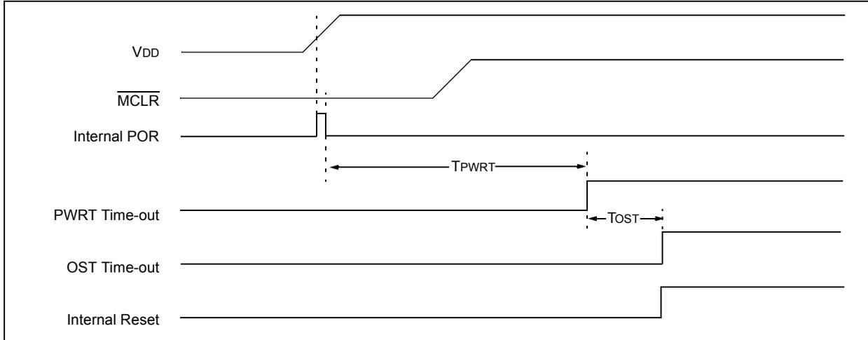
**FIGURE 14-5: TIME-OUT SEQUENCE ON POWER-UP (DELAYED  $\overline{\text{MCLR}}$ ): CASE 2**
