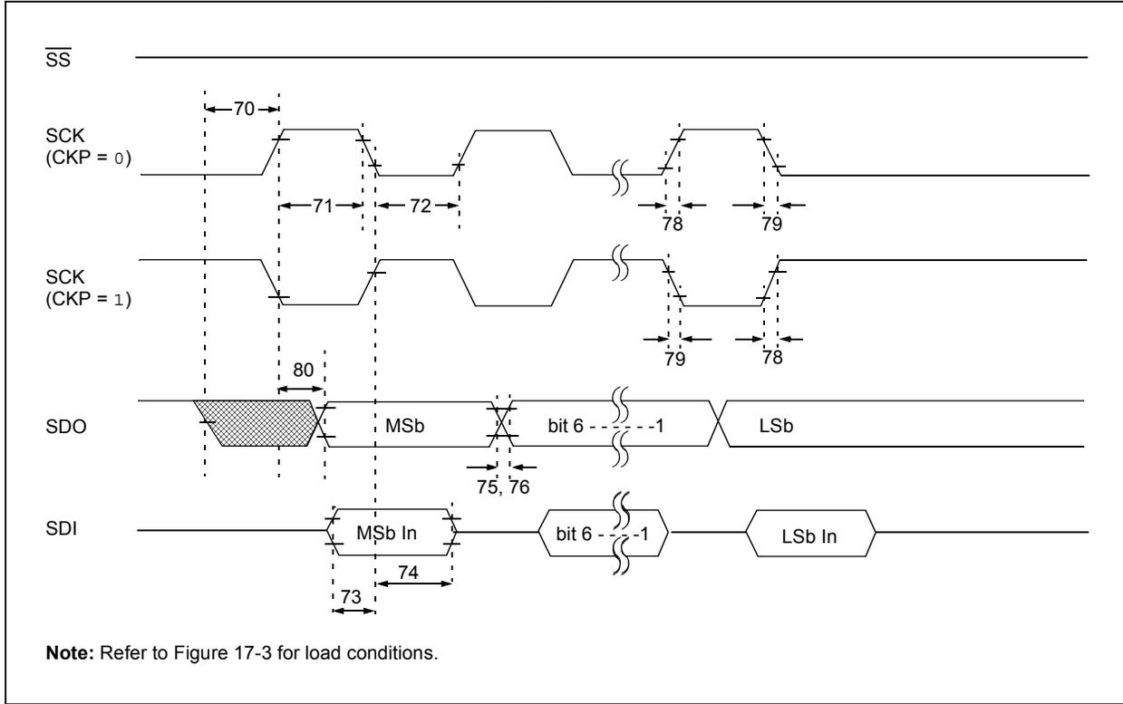
**FIGURE 17-13: SPI MASTER MODE TIMING (CKE = 1, SMP = 1)**
