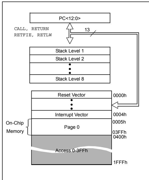
**FIGURE 2-2: PROGRAM MEMORY MAP AND STACK FOR THE PIC16F685/689/690**
