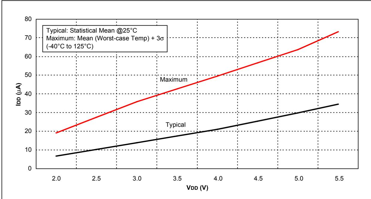
FIGURE 18-11: TYPICAL  $I_{DD}$  vs.  $F_{osc}$  OVER  $V_{DD}$  (HFINTOSC MODE)
