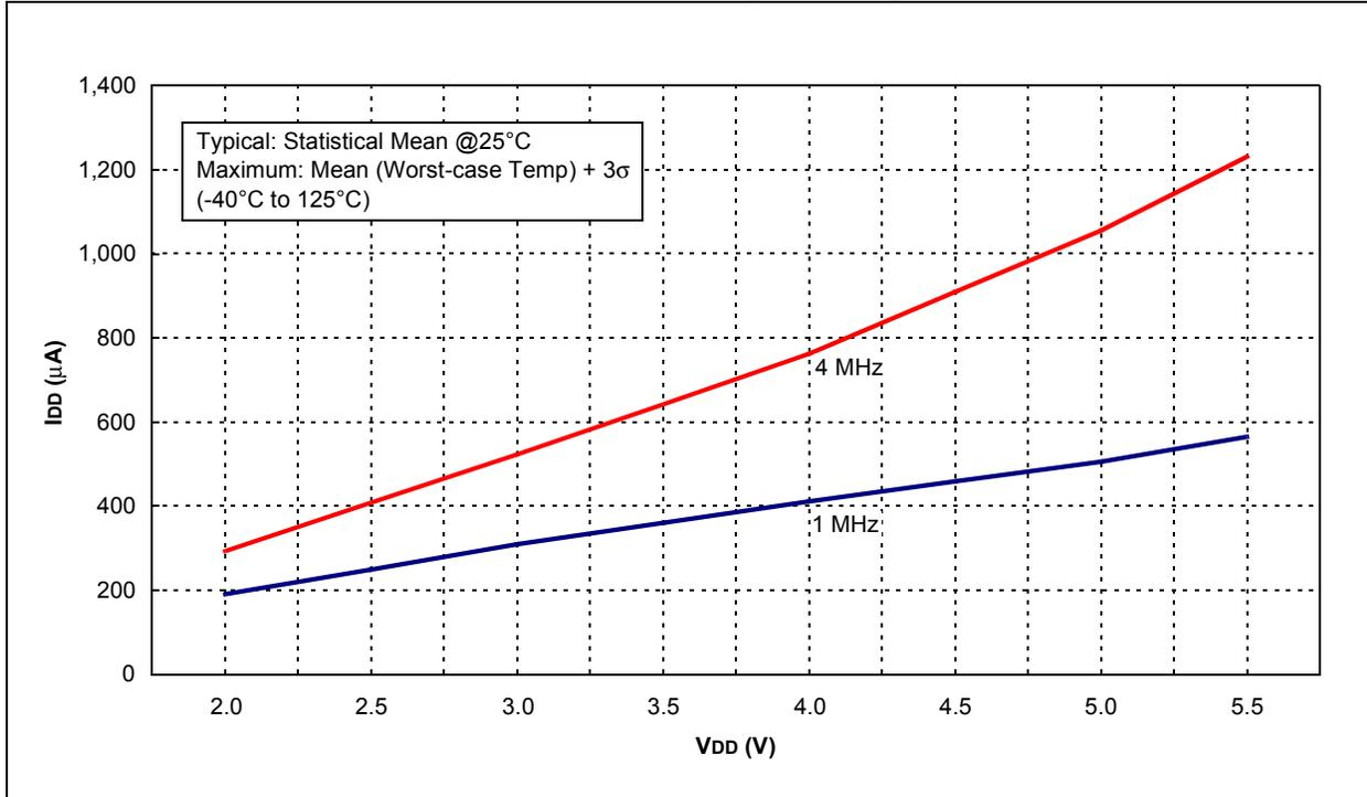
FIGURE 18-7:  $I_{DD}$  vs.  $V_{DD}$  (LP MODE)
