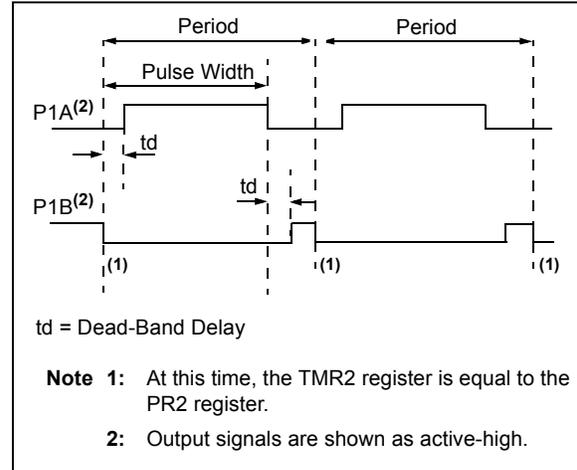
**FIGURE 11-18: EXAMPLE OF HALF-BRIDGE APPLICATIONS**
