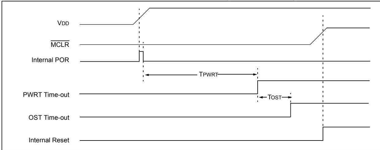
**FIGURE 14-6: TIME-OUT SEQUENCE ON POWER-UP ( $\overline{\text{MCLR}}$  WITH VDD)**
