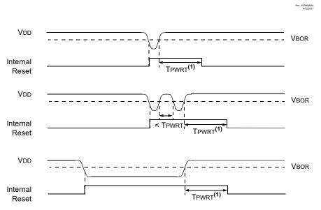
**Note:** T<sub>PWRT</sub> delay only if PWRTE bit is programmed to '0'.
