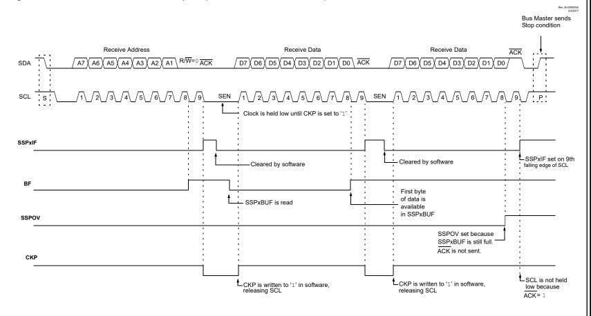
Figure 26-16. I<sup>2</sup>C Slave, 7-bit Address, Reception (SEN = 0, AHEN = 1, DHEN = 1)
