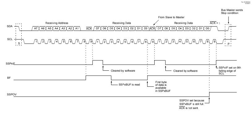
PIC18F24/25Q10 MSSP - Master Synchronous Serial Port Module
