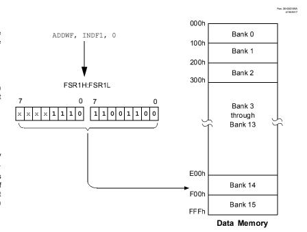
Operations on the FSRs with POSTDEC, POSTINC and PREINC affect the entire register pair; that is, rollovers of the FSRnL register from FFh to 00h carry over to the FSRnH register. On the other hand, results of these operations do not change the value of any flags in the STATUS register (e.g., Z, N, OV, etc.).
