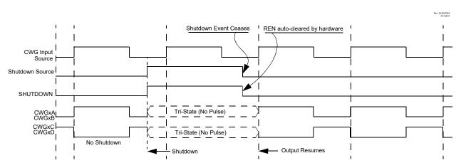
Figure 24-16. Shutdown Functionality, Auto-Restart Enabled (REN = 1, LSAC = 01, LSBD = 01)
