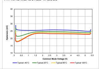
Figure 39-25. COMPARATOR OFFSET, NORMAL POWER MODE (CxSP = 1), Vdd = 5.5V, MEASURED VALUES AT 25°C
