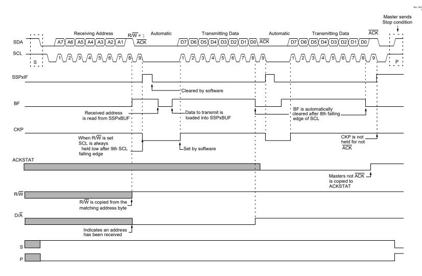
**MSSP - Master Synchronous Serial Port Module**
