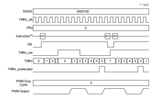
BSF and BCF represent Bit-Set File and Bit-Clear File instructions executed by the CPU to set or clear the ON bit of TxCON. CPU execution is asynchronous to the timer clock input.
