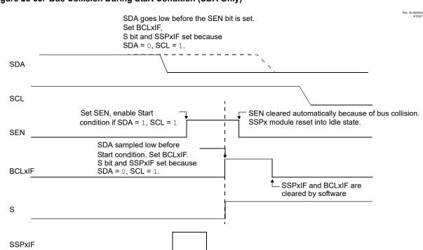
Figure 26-33. Bus Collision During Start Condition (SDA Only)
