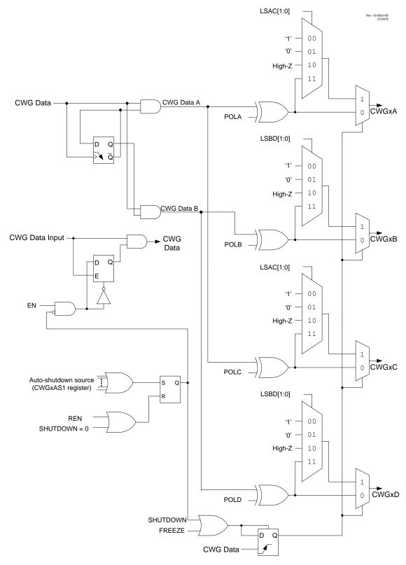
Figure 24-4. Simplified CWG Block Diagram (Push-Pull Mode, MODE[2:0] = 101)
