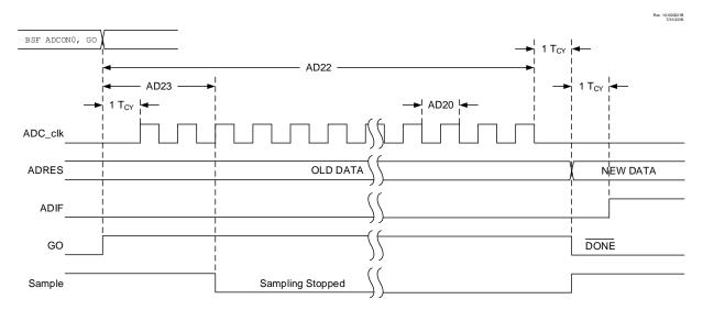
Figure 38-10. ADC Conversion Timing (ADC Clock from F<sub>RC</sub>)
