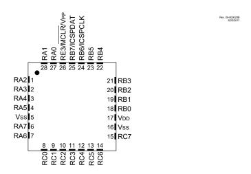
**Note:** It is recommended that the exposed bottom pad be connected to  $V_{SS}$ , however it must not be the only  $V_{SS}$  connection to the device.
