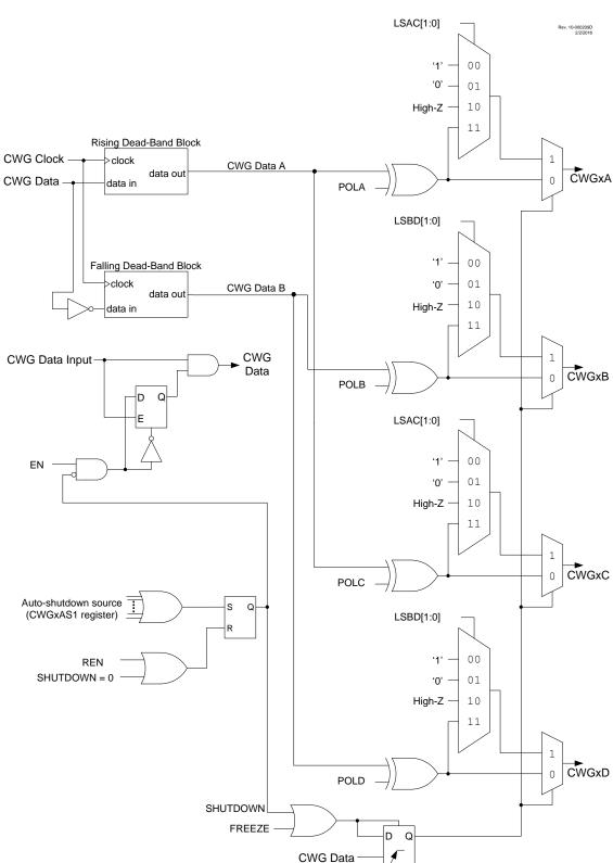
Figure 24-2. Simplified CWG Block Diagram (Half-Bridge Mode, MODE[2:0] = 100)
