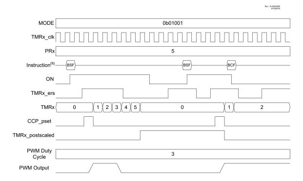
1. BSF and BCF represent Bit-Set File and Bit-Clear File instructions executed by the CPU to set or clear the ON bit of TxCON. CPU execution is asynchronous to the timer clock input.
