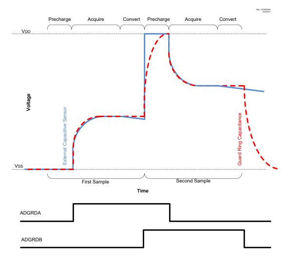
Figure 31-10. Hardware CVD Sequence Timing Diagram
