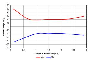
Figure 39-24. COMPARATOR HYSTERESIS, NORMAL POWER MODE (CxSP = 1), Vdd = 5.5V, TYPICAL MEASURED VALUES
