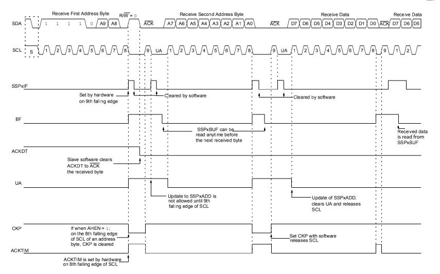
Figure 26-22.  $I^2C$  Slave, 10-bit Address, Transmission (SEN = 0, AHEN = 0, DHEN = 0)
