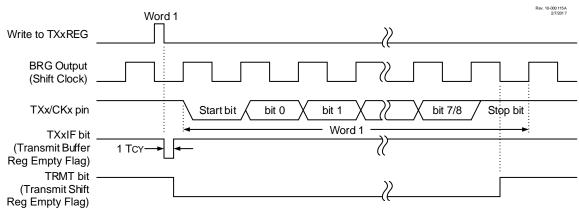
Figure 27-4. Asynchronous Transmission (Back-to-Back)
