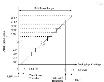
Figure 31-5. ADC Transfer Function
