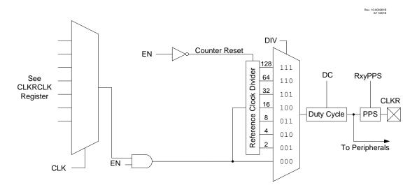
Figure 5-2. Clock Reference Timing
