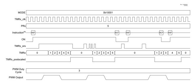
1. BSF and BCF represent Bit-Set File and Bit-Clear File instructions executed by the CPU to set or clear the ON bit of TxCON. CPU execution is asynchronous to the timer clock input.
