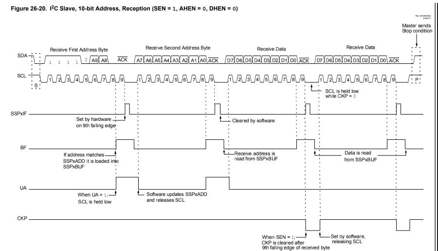
PIC18F24/25Q10 MSSP - Master Synchronous Serial Port Module
