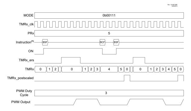
1. BSF and BCF represent Bit-Set File and Bit-Clear File instructions executed by the CPU to set or clear the ON bit of TxCON. CPU execution is asynchronous to the timer clock input.
