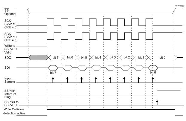
Figure 26-7. SPI Mode Waveform (Slave Mode with CKE = 0)
