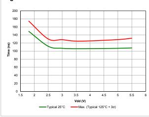
Figure 39-28. Comparator Response Time Rising edge
