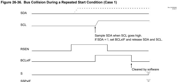
If SCL goes from high-to-low before the BRG times out and SDA has not already been asserted, a bus collision occurs. In this case, another master is attempting to transmit a data '1' during the Repeated Start condition, see Figure 26-37.
