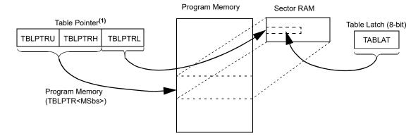
Note 1: During table writes the Table Pointer points to two areas. The LSbs of TBLPRTL point to an address within the sector RAM space. The MSbs of the Table Pointer determine where the sector will eventually be written.
