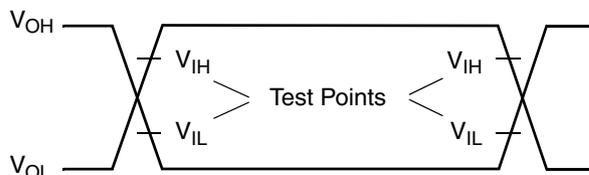
Figure 8. AC Test Conditions,  $T_A = 0^{\circ}\text{C} \text{ to } 70^{\circ}\text{C}$ ,  $V_{SUP} = 3.13\text{V} - 3.47\text{V}$
