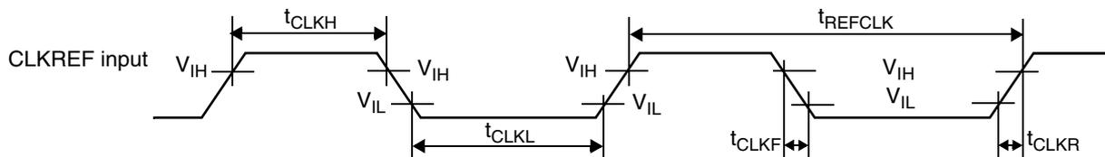
Figure 12. CLKREF Clock Waveforms
