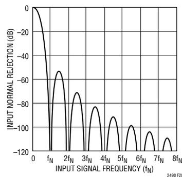
Figure 28. Input Normal Mode Rejection 2x Speed Mode
