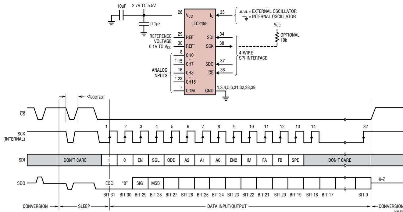
Figure 9. Internal Serial Clock, Single Cycle Operation
