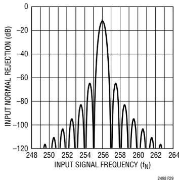
Figure 29. Input Normal Mode Rejection 2x Speed Mode
