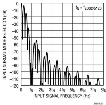
Figure 21. Input Normal Mode Rejection at DC
