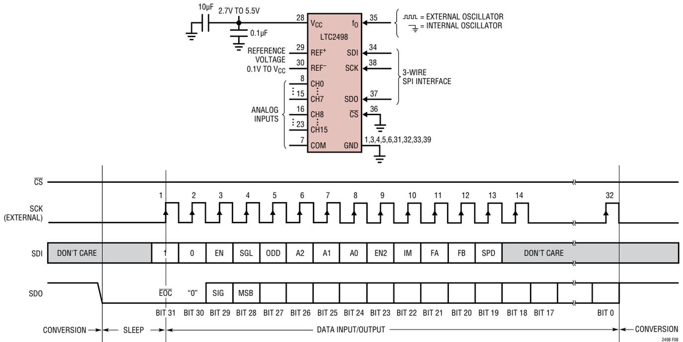
Figure 8. External Serial Clock, 3-Wire Operation ( $\overline{CS} = 0$ )
