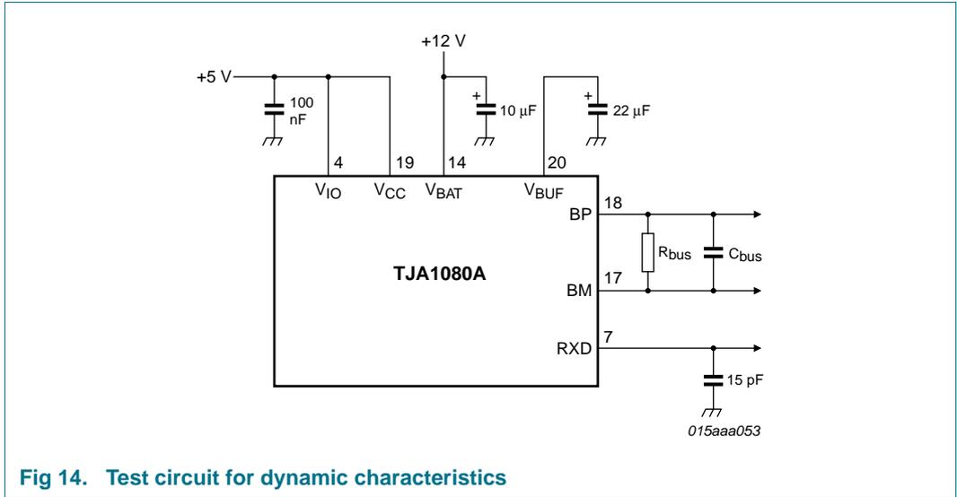
Fig 14. Test circuit for dynamic characteristics
