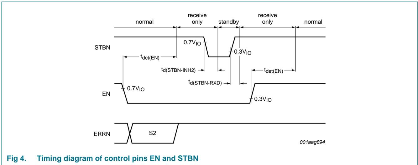
Fig 4. Timing diagram of control pins EN and STBN
