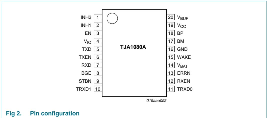
Fig 2. Pin configuration
