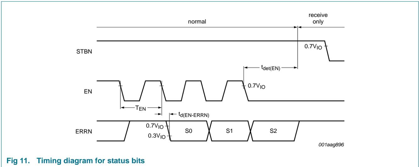
Fig 11. Timing diagram for status bits
