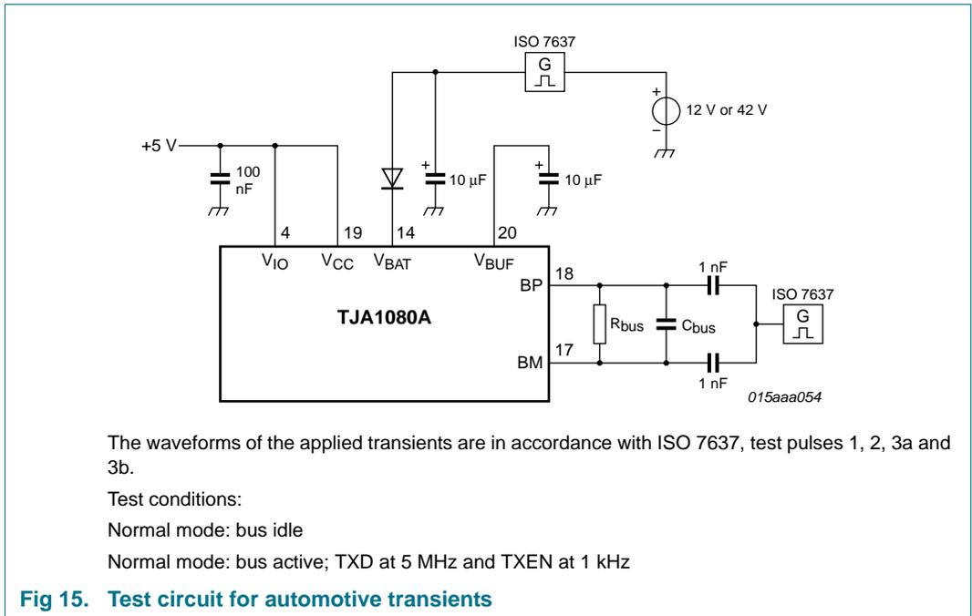
The waveforms of the applied transients are in accordance with ISO 7637, test pulses 1, 2, 3a and 3b.
