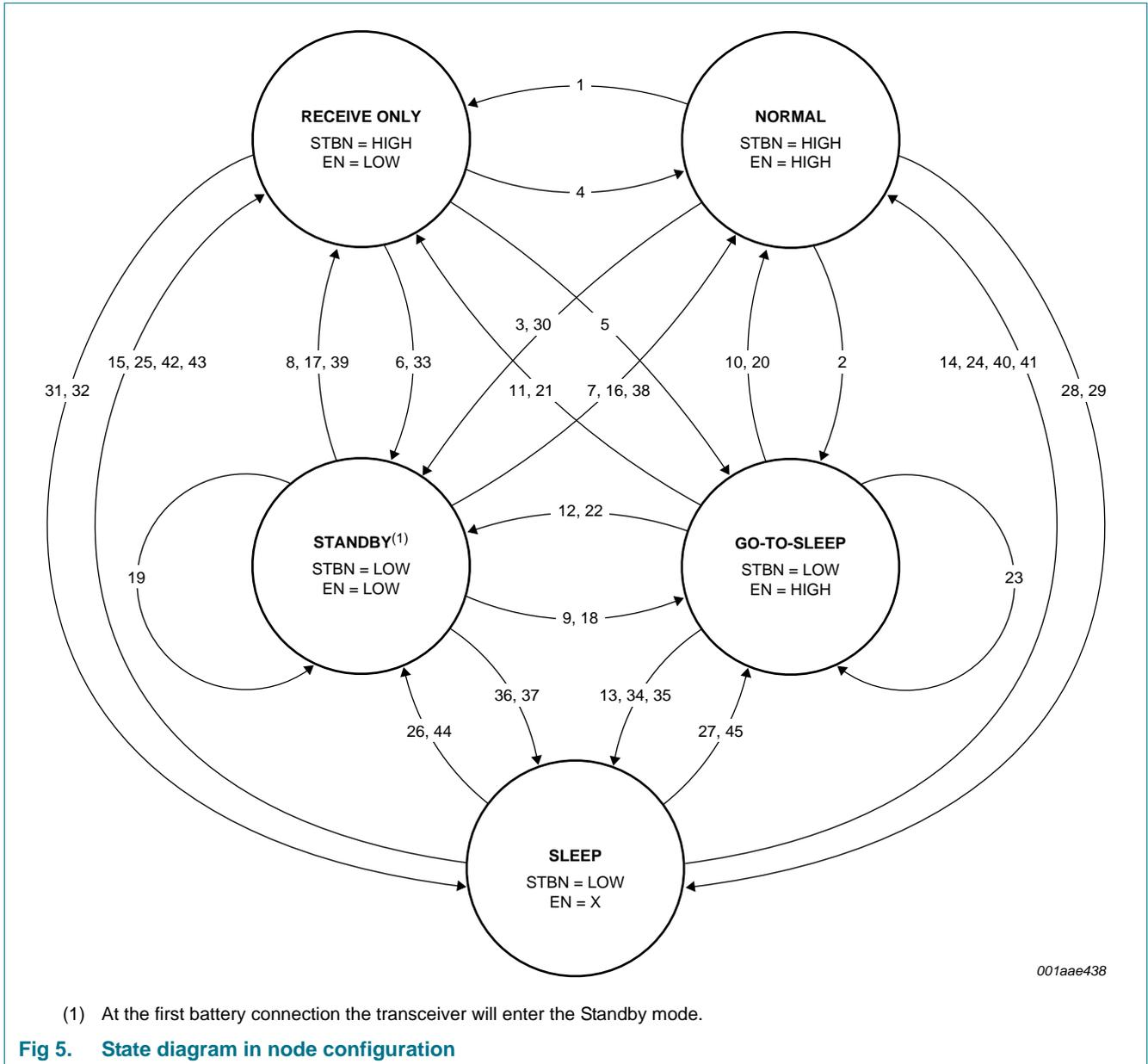
The state transitions are represented with numbers, which correspond with the numbers in column 3 of [Table 4](#) to [Table 7](#).
