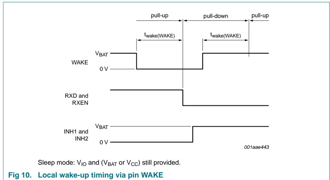
**Fig 10. Local wake-up timing via pin WAKE**
