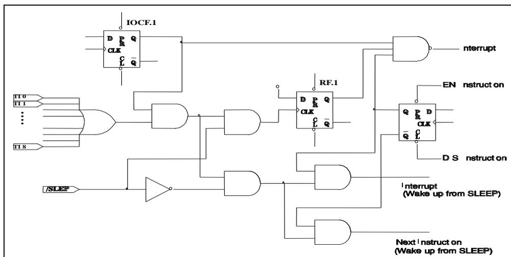
Figure 6-7 Port 5 Block Diagram with Input Change Interrupt/Wake-up
