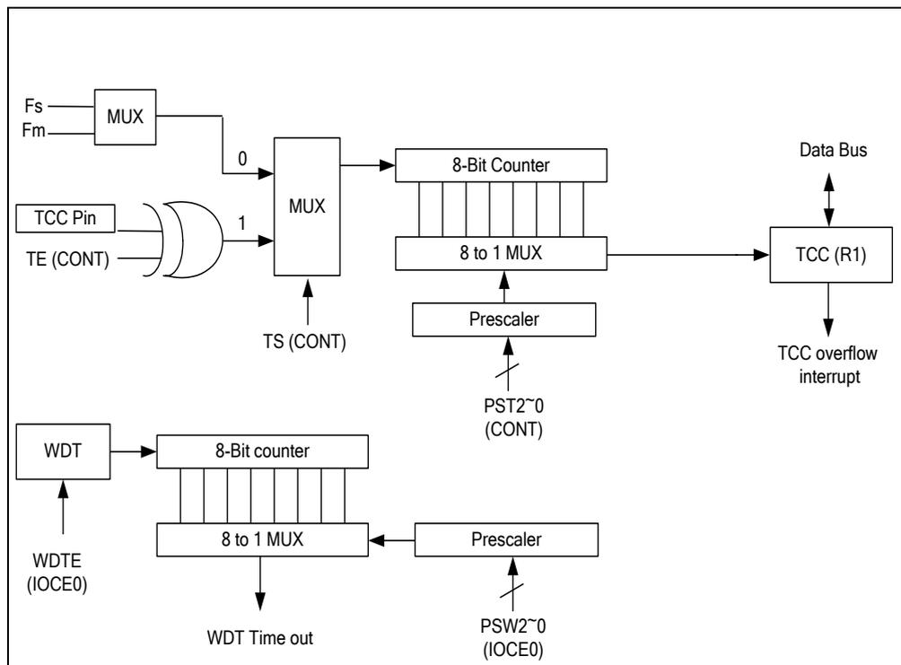
Figure 6-3 TCC and WDT Block Diagram
