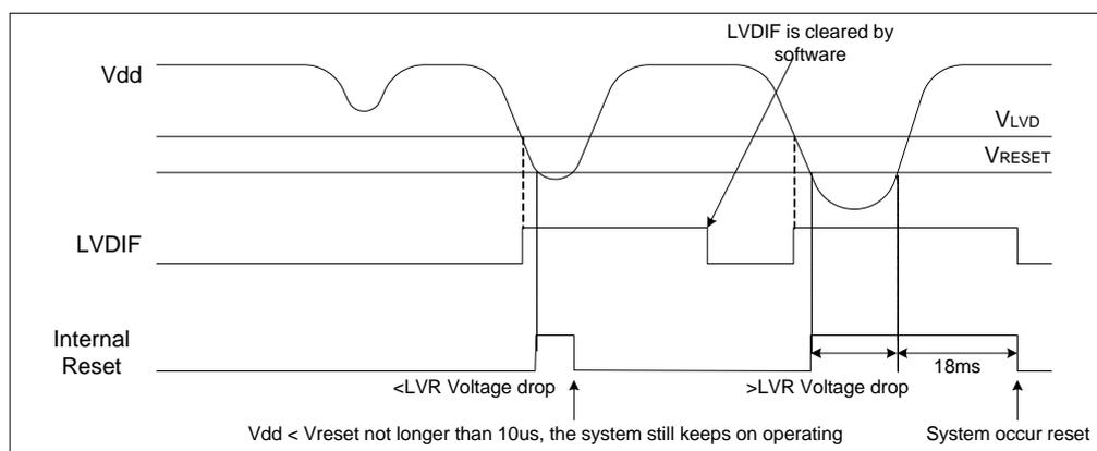
Figure 6-26 LVD/LVR Waveform
