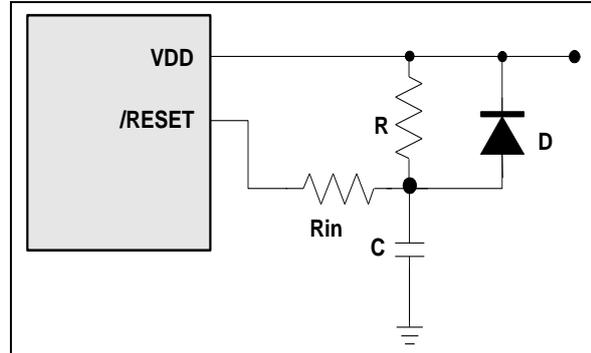
Figure 6-23 External Power-on Reset Circuit
