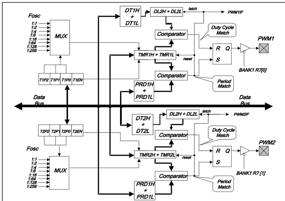
Figure 6-12 PWM System Block Diagram
