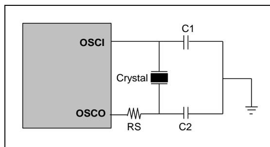
Figure 6-18 Crystal/Resonator Circuit
