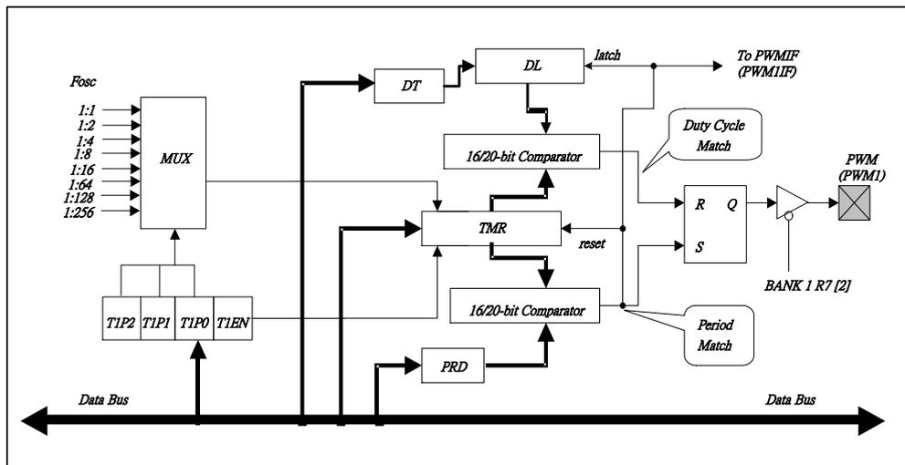
Figure 6-14 Functional Block Diagram of 16/20-bit PWM (merged from two 8/10 bits)
