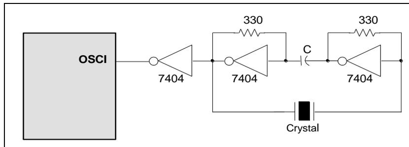
Figure 6-19 Serial Mode Crystal/Resonator Circuit Diagram
