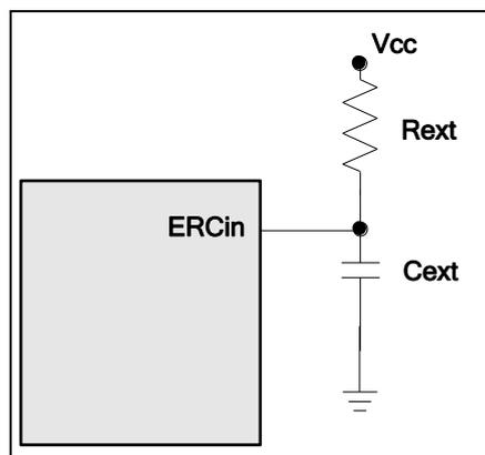
Figure 6-22 External RC Oscillator Mode Circuit
