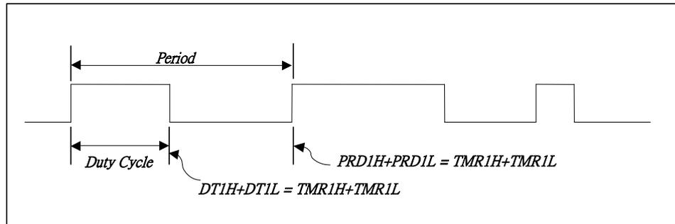
Figure 6-13 PWM Output Timing
