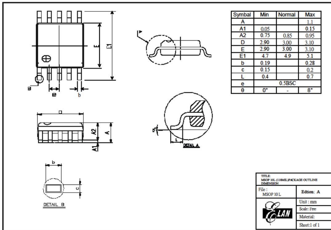
Figure C-9 EM78P301N 10-pin MSOP Package Type
