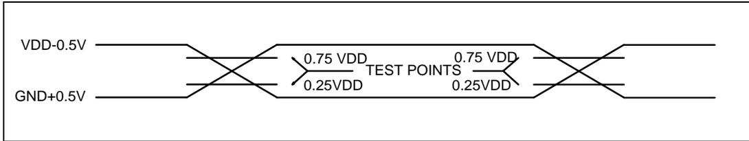
**Note:** AC Testing: Input is driven at VDD-0.5V for logic "1", and GND+0.5V for Logic "0"
