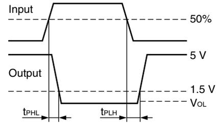
CL is approximately 15 pF which includes probe and stray wiring capacitance.
