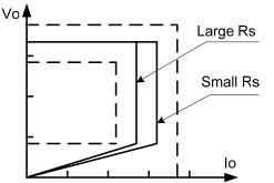
Figure.3. Adjustable output power by changing Rs
