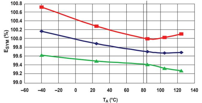
Total Output Error versus Ambient Temperature
