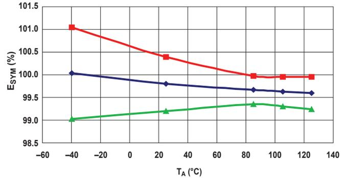
Total Output Error versus Ambient Temperature
