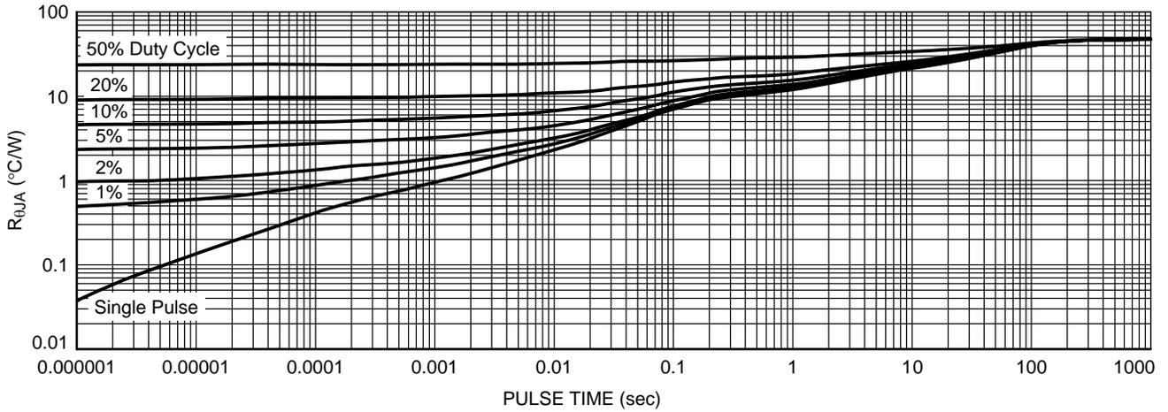
Figure 13. Thermal Characteristics
