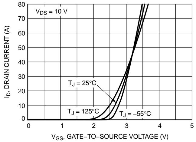
Figure 2. Transfer Characteristics
