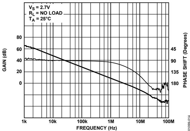
Figure 14. Open-Loop Gain and Phase Shift vs. Frequency
