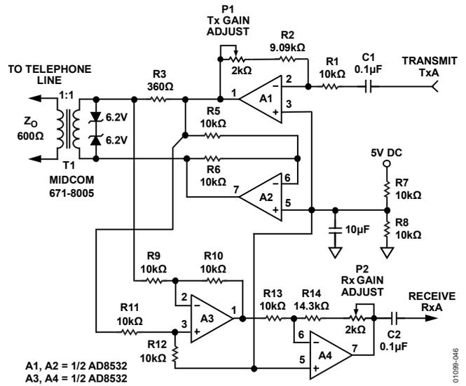
Figure 46. Single-Supply Direct Access Arrangement for Modems
