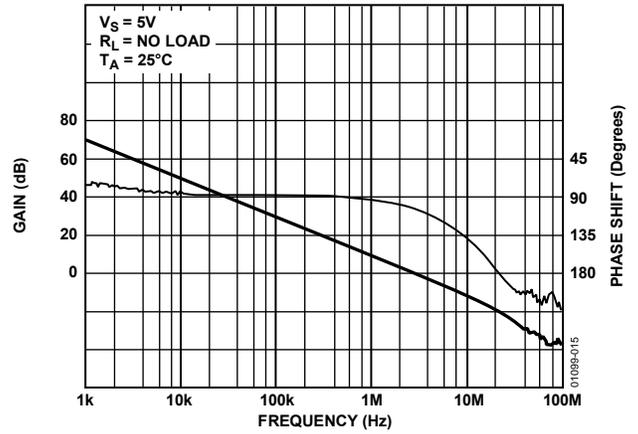
Figure 15. Open-Loop Gain and Phase Shift vs. Frequency
