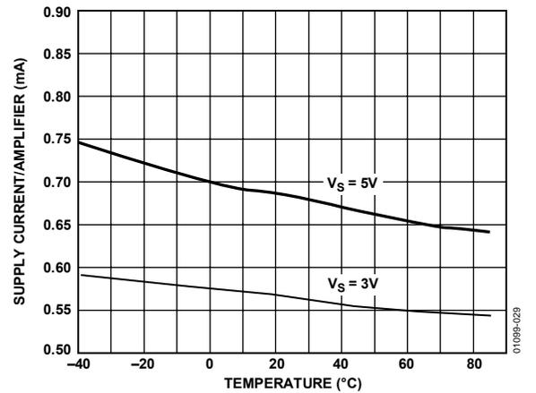
Figure 29. Supply Current per Amplifier vs. Temperature
