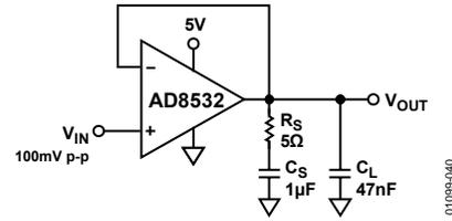
Figure 40. Snubber Network Compensates for Capacitive Loads
