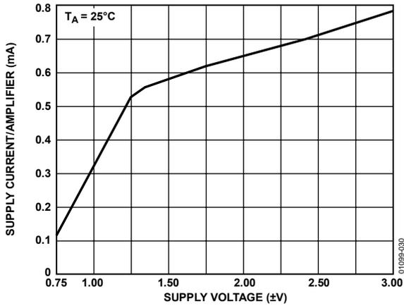
Figure 30. Supply Current per Amplifier vs. Supply Voltage
