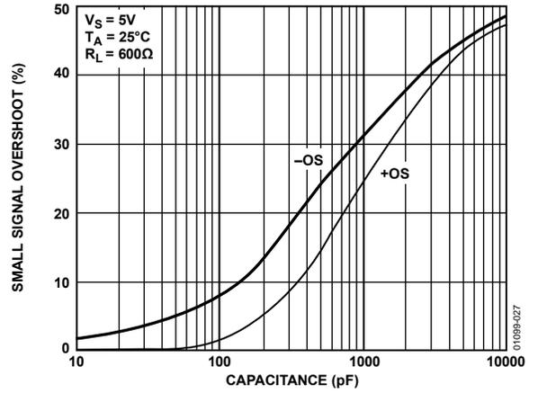
Figure 27. Small Signal Overshoot vs. Load Capacitance
