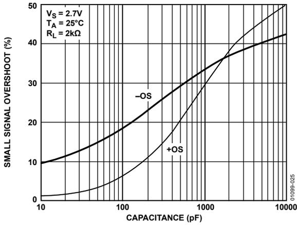
Figure 25. Small Signal Overshoot vs. Load Capacitance
