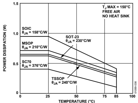
Figure 38. Maximum Power Dissipation vs. Ambient Temperature
