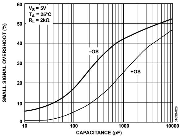
Figure 26. Small Signal Overshoot vs. Load Capacitance
