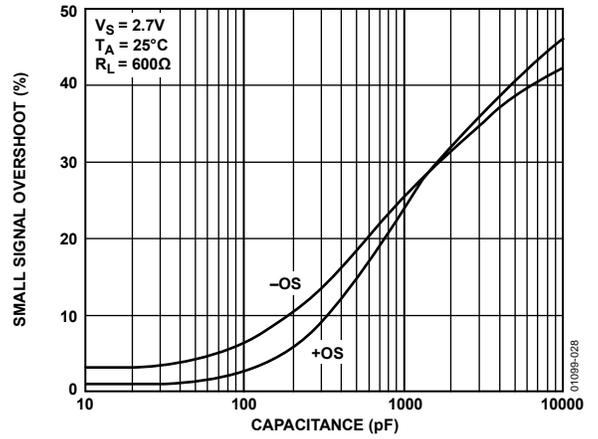
Figure 28. Small Signal Overshoot vs. Load Capacitance
