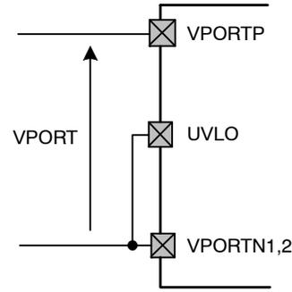
**Figure 5. Default Internal UVLO Configuration (NCP1091 only)**
