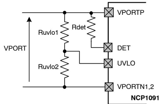
**Figure 6. Default Internal UVLO Configuration (NCP1091 only)**
