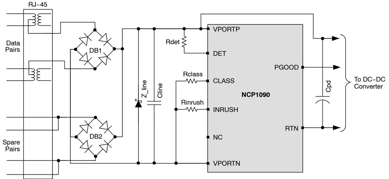
Figure 2. Typical Application Circuit using the NCP1090
