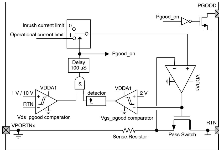
**Figure 7. Inrush and Operational Current Limitation Selection Mechanism**
