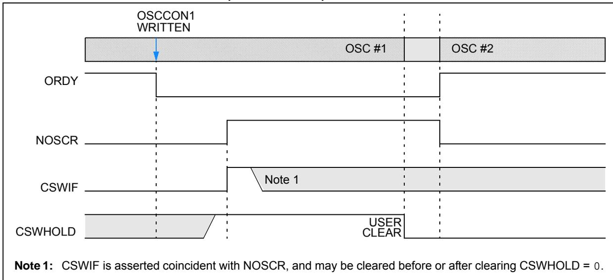
**FIGURE 7-8: CLOCK SWITCH ABANDONED**
