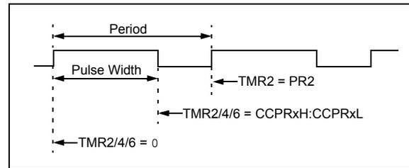
**FIGURE 29-4: SIMPLIFIED PWM BLOCK DIAGRAM**
