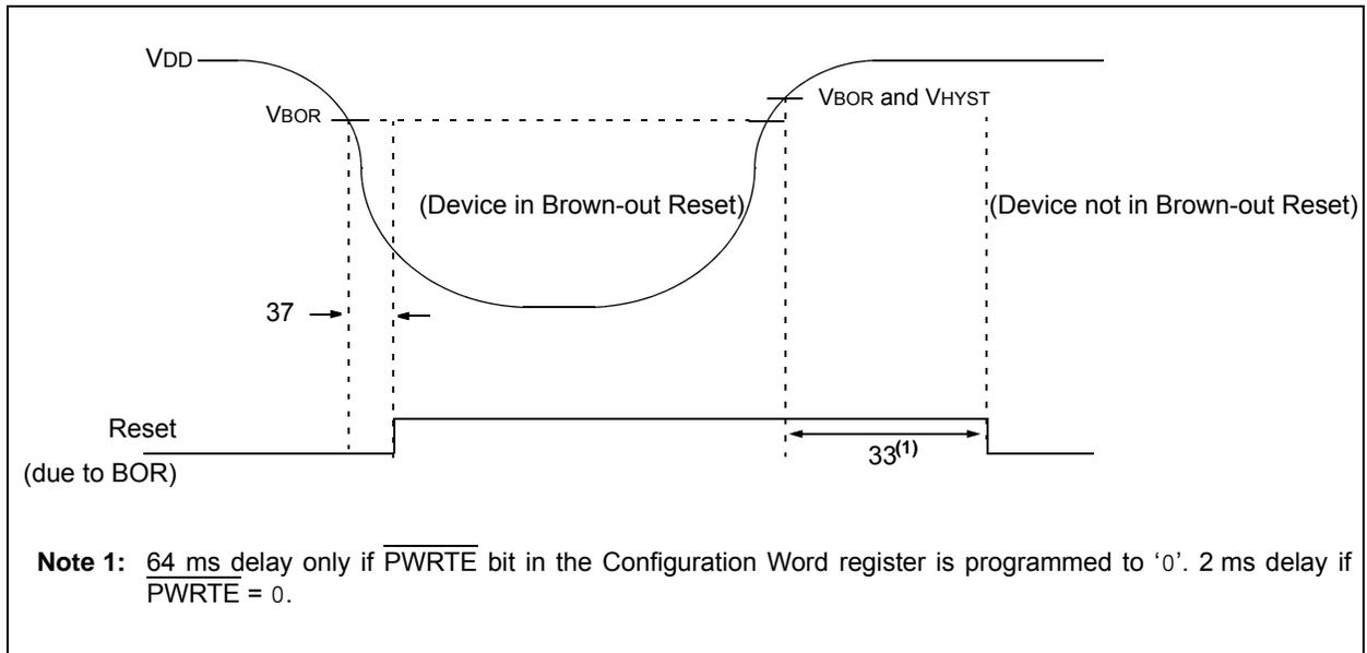
**Note 1:** 64 ms delay only if  $\overline{\text{PWRTE}}$  bit in the Configuration Word register is programmed to '0'. 2 ms delay if  $\overline{\text{PWRTE}} = 0$ .
