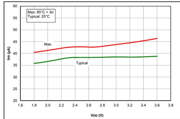
**FIGURE 36-16:** *IPD, Fixed Voltage Reference (FVR), PIC16LF18313/18323 Only*
