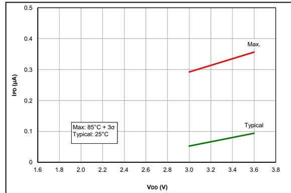
**FIGURE 36-20:** *IPD, Low-Power Brown-out Reset (LPBOR = 0), PIC16LF18313/18323 Only*
