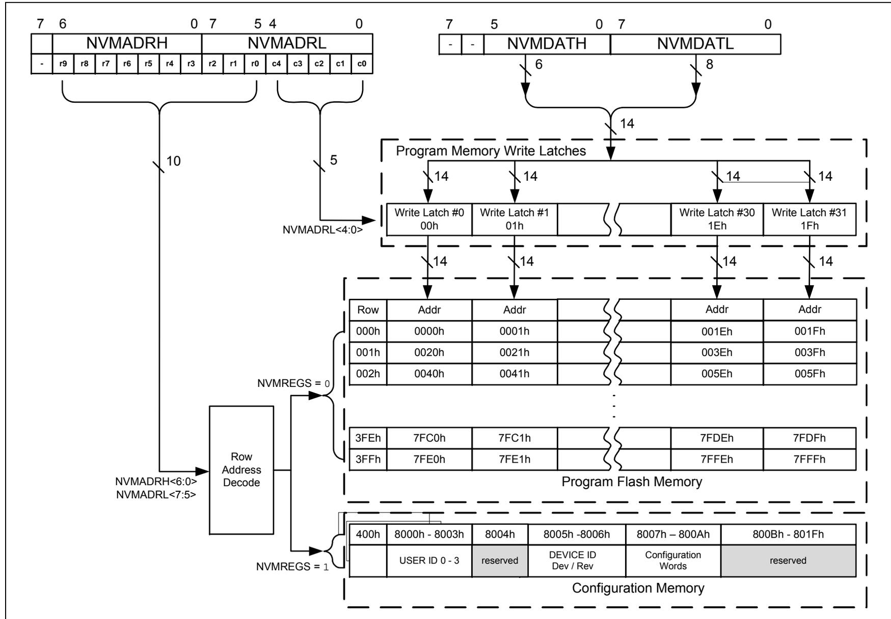
**FIGURE 11-5: PROGRAM FLASH MEMORY WRITE FLOWCHART**
