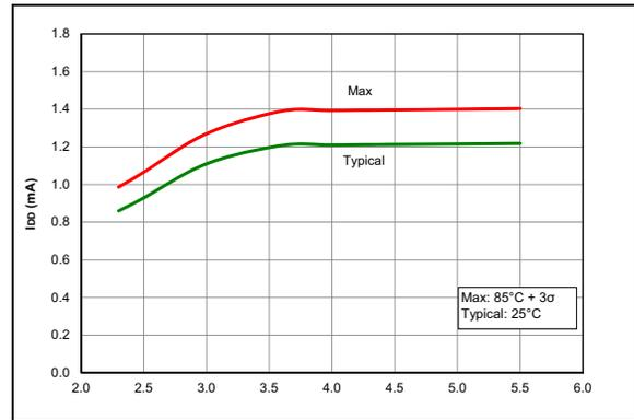
**FIGURE 36-8:**  $I_{DD}$ , HFINTOSC Mode,  $F_{OSC} = 16$  MHz, PIC16F18313/18323 Only
