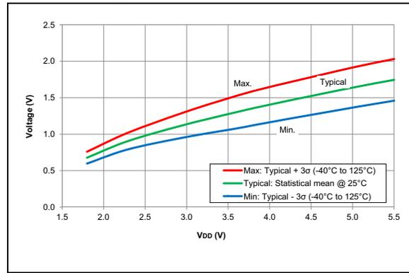
**FIGURE 36-98:** Schmitt Trigger Low Values, All devices
