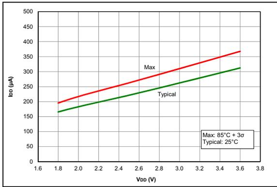
**FIGURE 36-1:**  $I_{DD}$ , XT Oscillator, 4 MHz, PIC16LF18313/18323 Only
