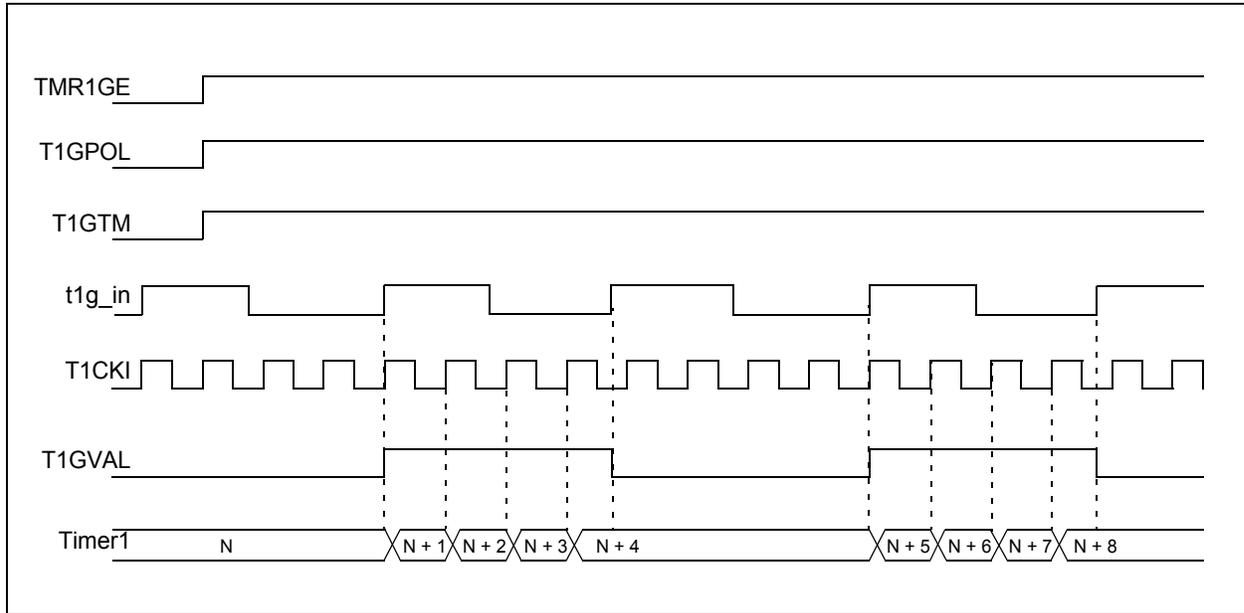
**FIGURE 27-5: TIMER1 GATE SINGLE-PULSE MODE**
