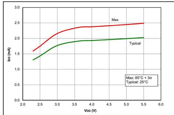
**FIGURE 36-4:**  $I_{DD}$ , HS Oscillator, 32 MHz, PIC16F18313/18323 Only
