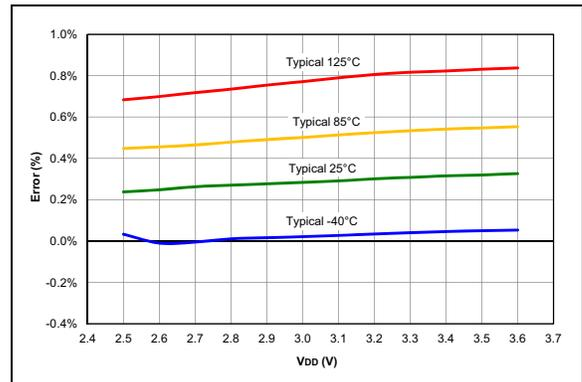
**FIGURE 36-94:** FVR Voltage Error (2x), PIC16LF18313/18323 Only
