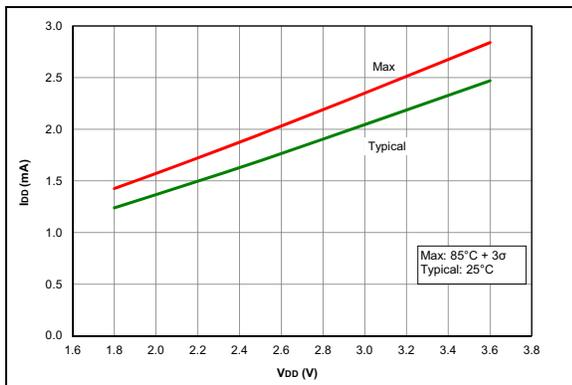
**FIGURE 36-5:**  $I_{DD}$ , HFINTOSC Mode, FOSC = 32 MHz, PIC16LF18313/18323 Only
