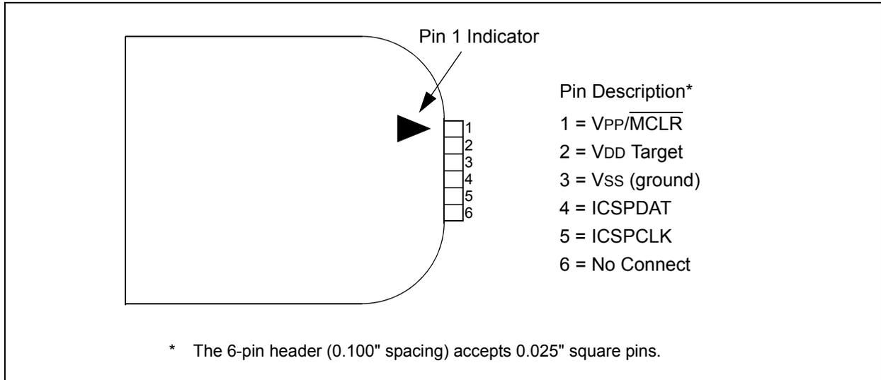
**FIGURE 33-3: TYPICAL CONNECTION FOR ICSP™ PROGRAMMING**
