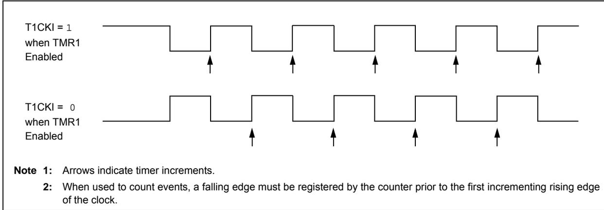
**FIGURE 27-3: TIMER1 GATE ENABLE MODE**
