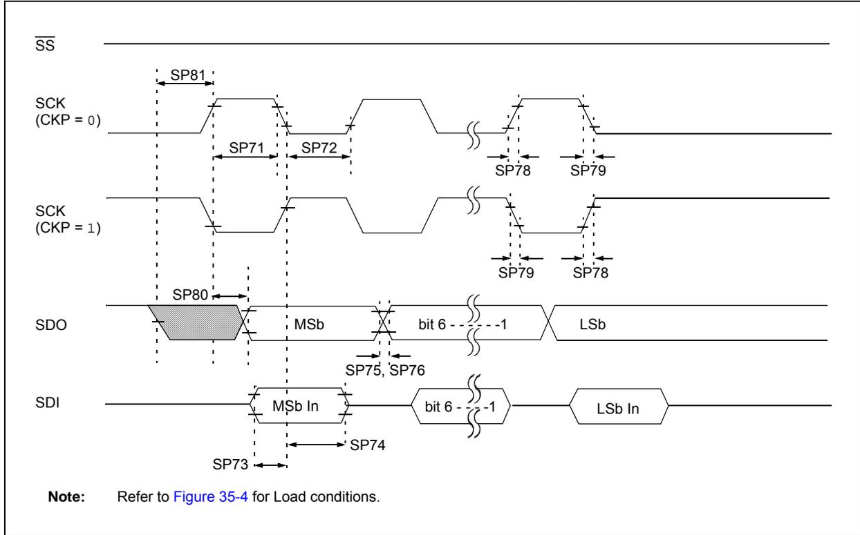
**FIGURE 35-18: SPI MASTER MODE TIMING (CKE = 1, SMP = 1)**
