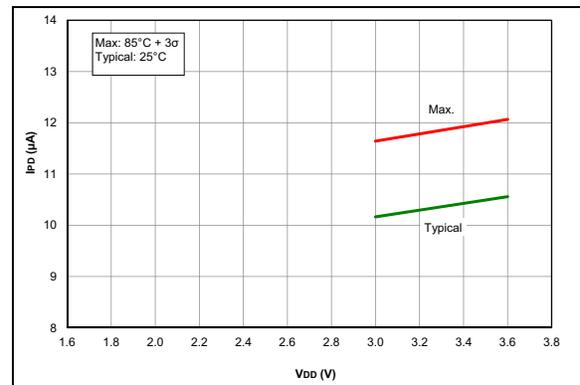
**FIGURE 36-18:** *IPD, Brown-out Reset (BOR), BORV = 1, PIC16LF18313/18323 Only*
