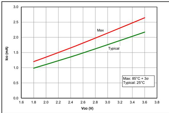
**FIGURE 36-3:**  $I_{DD}$ , HS Oscillator, 32 MHz, PIC16LF18313/18323 Only
