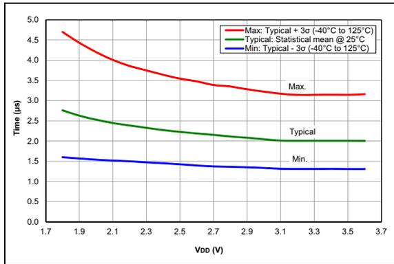
**FIGURE 36-67:** ADC RC Oscillator period, PIC16LF18313/18323 Only
