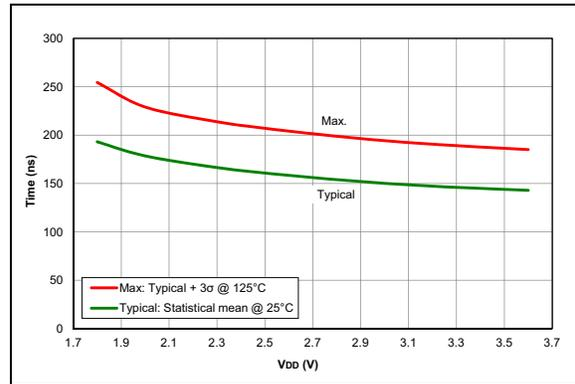
**FIGURE 36-86:** Comparator Response Time Falling edge, PIC16LF18313/18323 Only
