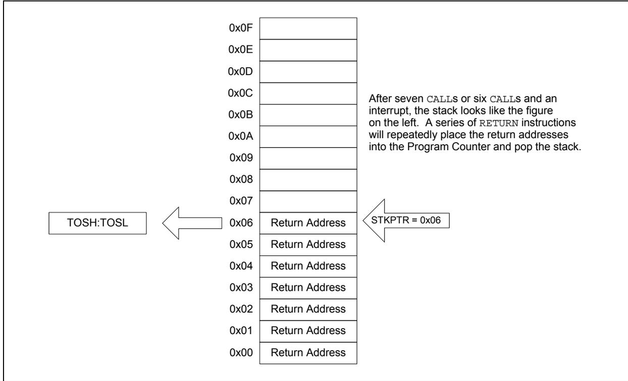
**FIGURE 4-7: ACCESSING THE STACK EXAMPLE 4**
