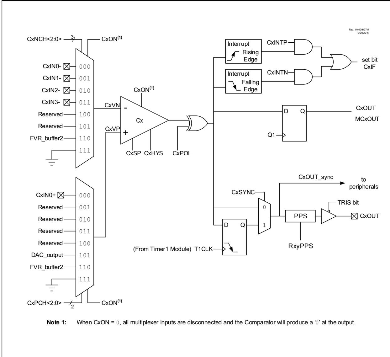
**Note 1:** When CxON = 0, all multiplexer inputs are disconnected and the Comparator will produce a '0' at the output.
