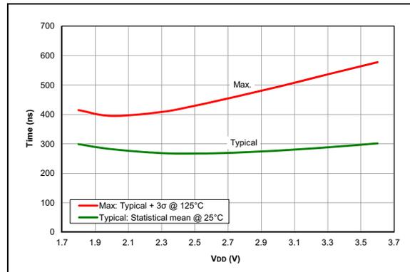
**FIGURE 36-88:** Comparator Response Time Rising edge, PIC16F18313/18323 Only
