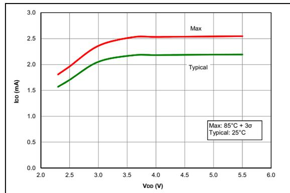
**FIGURE 36-6:**  $I_{DD}$ , HFINTOSC Mode, FOSC = 32 MHz, PIC16F18313/18323 Only
