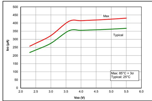
**FIGURE 36-2:**  $I_{DD}$ , XT Oscillator, 4 MHz, PIC16F18313/18323 Only
