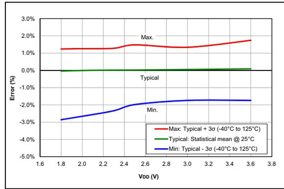
**FIGURE 36-26:** HFINTOSC Typical Frequency Error, PIC16LF18313/18323 Only
