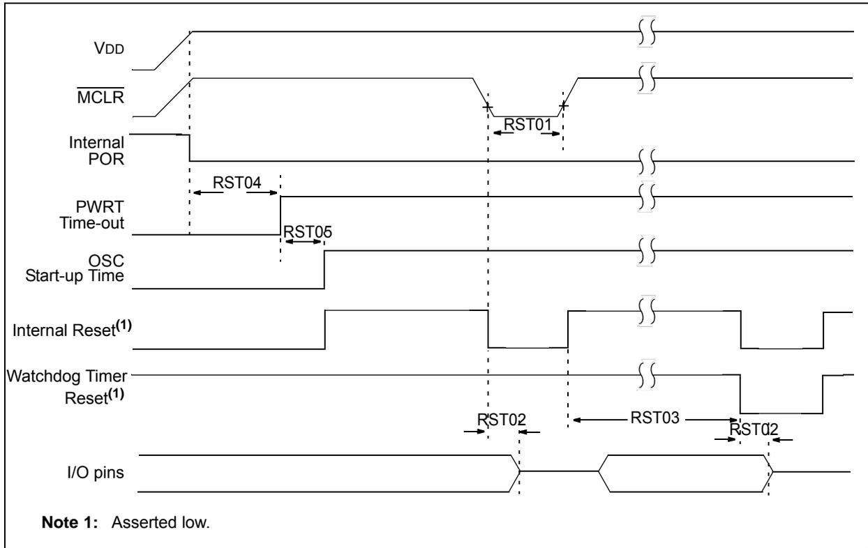
**FIGURE 35-9: BROWN-OUT RESET TIMING AND CHARACTERISTICS**
