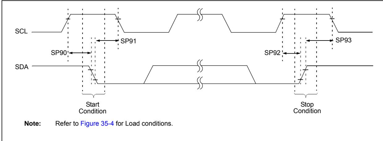
**TABLE 35-23: I<sup>2</sup>C BUS START/STOP BITS CHARACTERISTICS**
