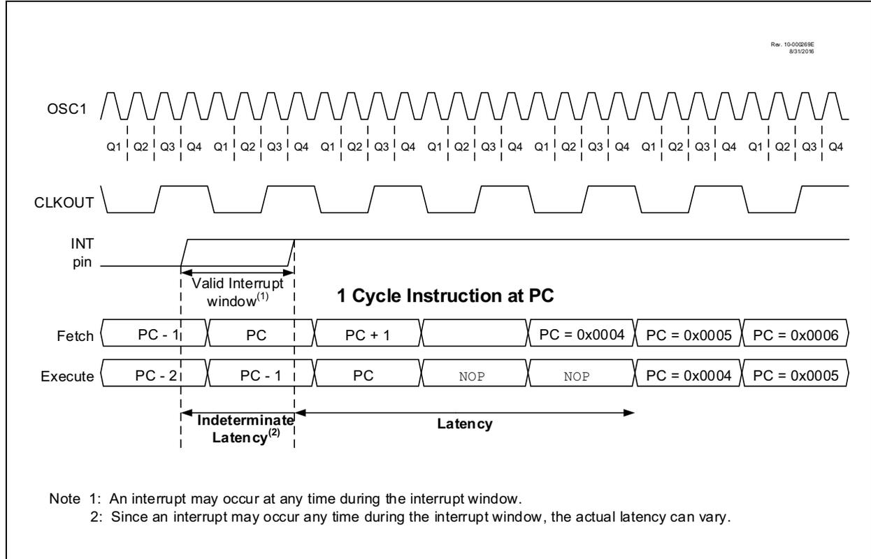
**FIGURE 8-3: INT PIN INTERRUPT TIMING**
