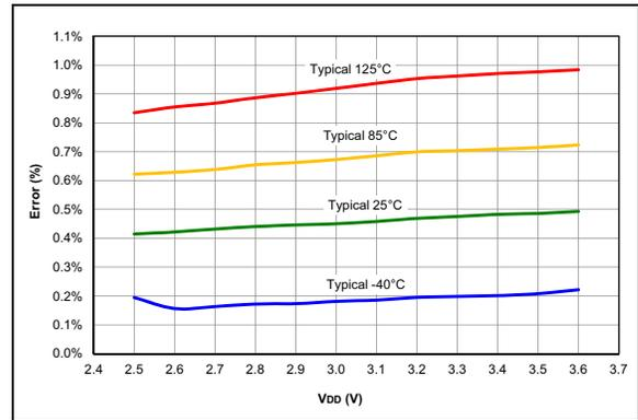
**FIGURE 36-92:** Typical FVR Voltage (1x), PIC16LF18313/18323 Only
