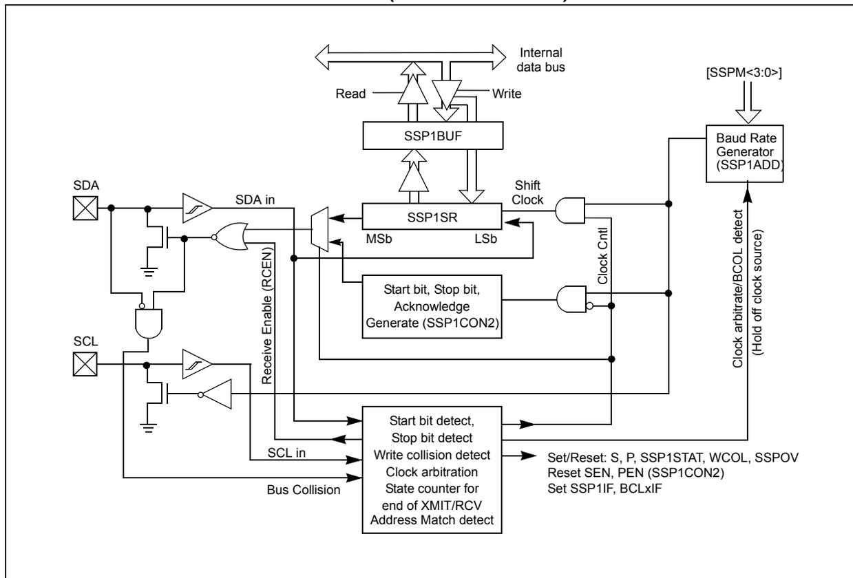
**FIGURE 30-3: MSSP BLOCK DIAGRAM (I<sup>2</sup>C SLAVE MODE)**
