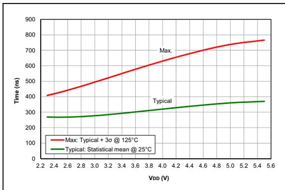
**FIGURE 36-89:** Comparator Response Time Rising edge, PIC16F18313/18323 Only
