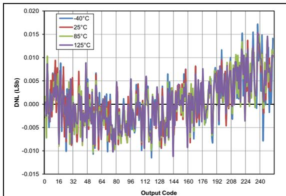
**FIGURE 36-71:** Typical DAC DNL Error, VDD = 5.0V, VREF = External 5V, PIC16F18313/18323 Only
