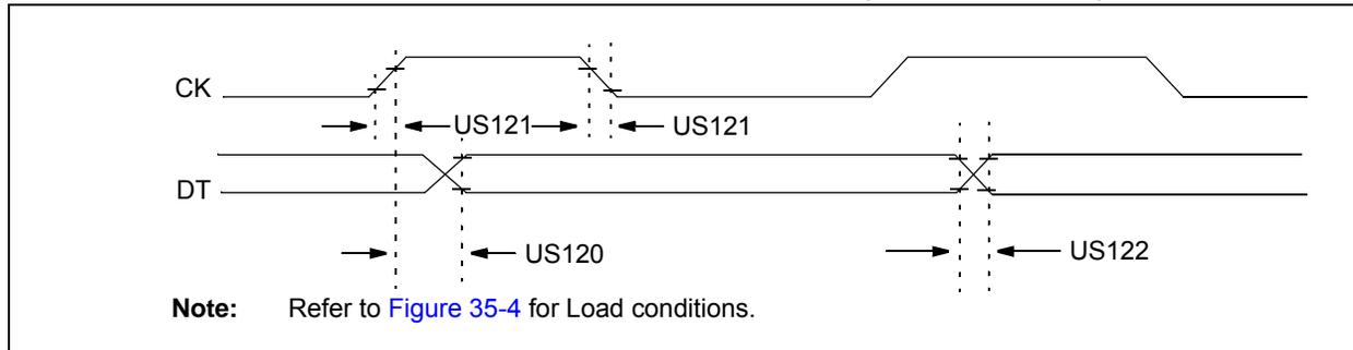
**TABLE 35-20: EUSART SYNCHRONOUS TRANSMISSION CHARACTERISTICS**
