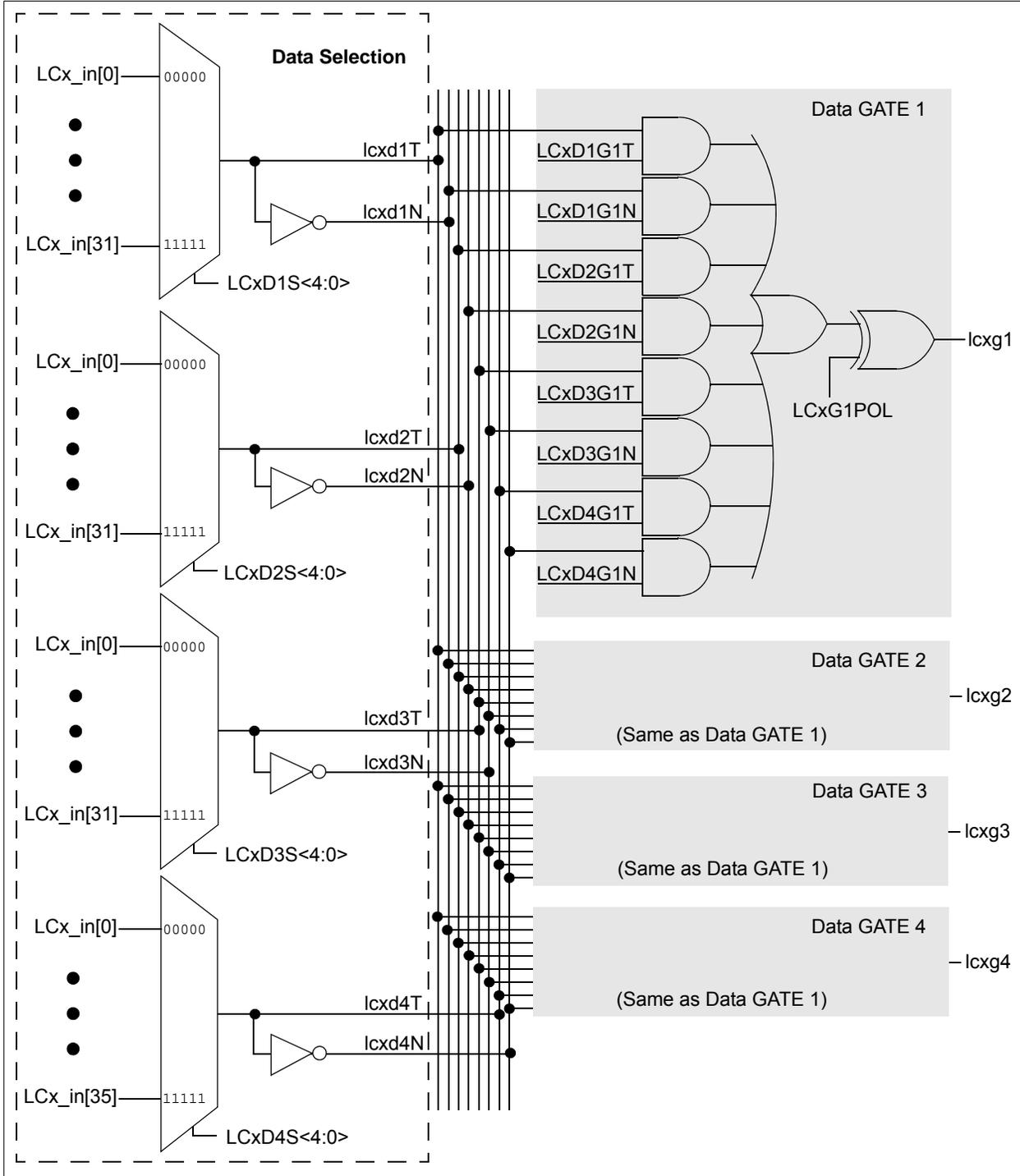
**FIGURE 21-3: PROGRAMMABLE LOGIC FUNCTIONS**
