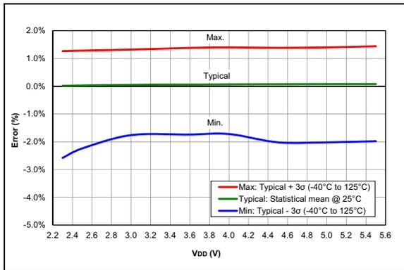
**FIGURE 36-27:** HFINTOSC Typical Frequency Error, PIC16F18313/18323 Only
