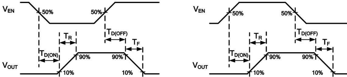
Figure 1. Voltage Waveforms: AP2101 (left), AP2111 (right)
