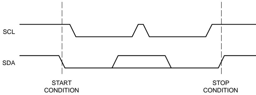
**Figure 2. Start/Stop Timing**
