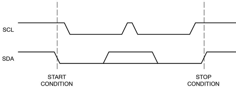
Figure 2. Start/Stop Timing
