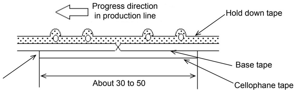
No lifting for the direction of progressing
