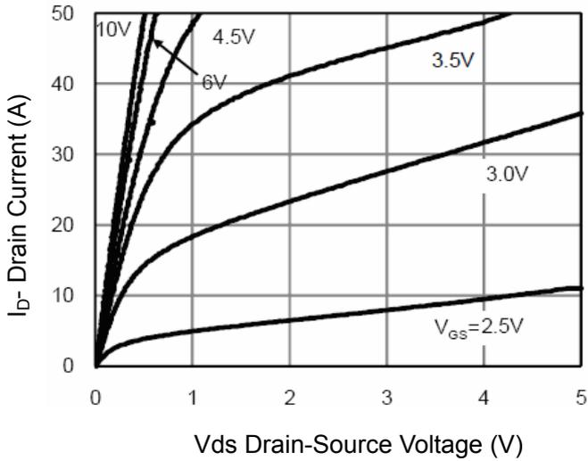
**Figure 1 Output Characteristics**
