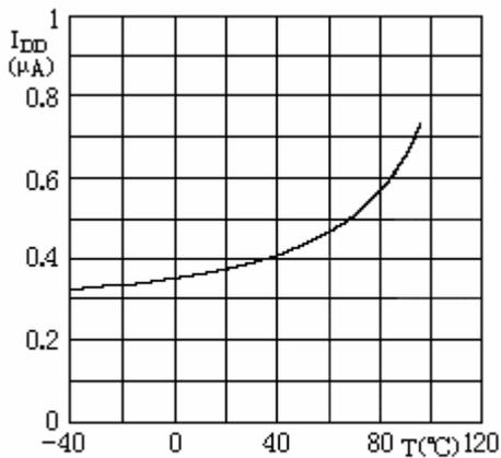
$V_{DD}=3\text{V}$ , Timer=1 minute
