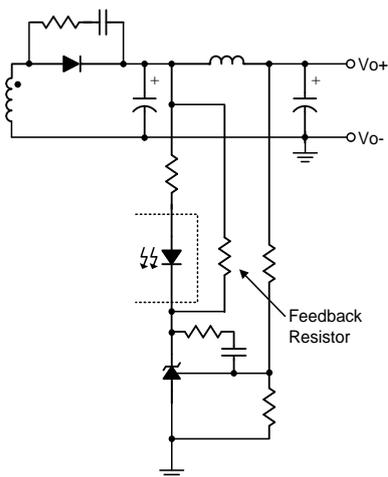
Figure 10. Feedback Resistor
