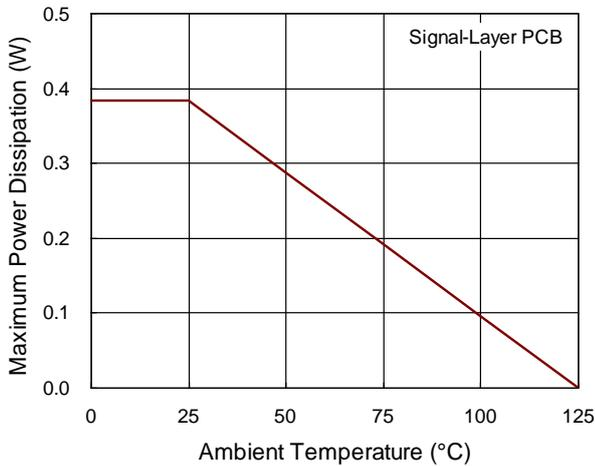
Figure 12. Derating Curve of Maximum Power Dissipation
