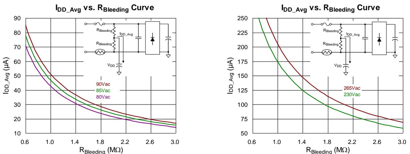
Figure 7. I<sub>DD\_Avg</sub> vs. R<sub>Bleeding</sub> Curve
