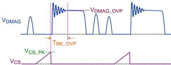
Figure 6. Resonance Waveform on the DMAG Pin
