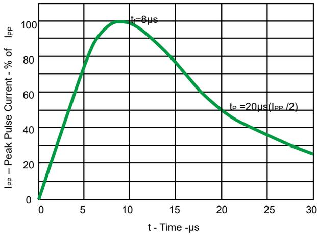
Fig 1. Pulse Waveform
