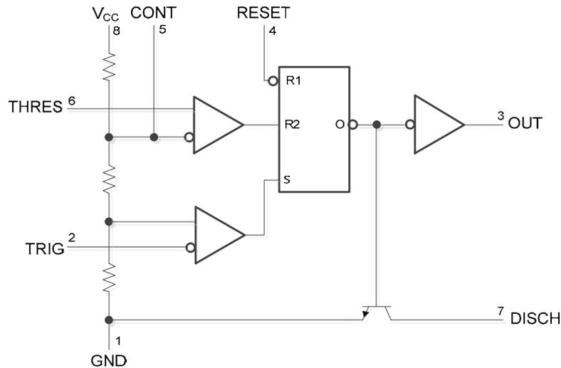
**RESET can override TRIG, which can override THRESH**
