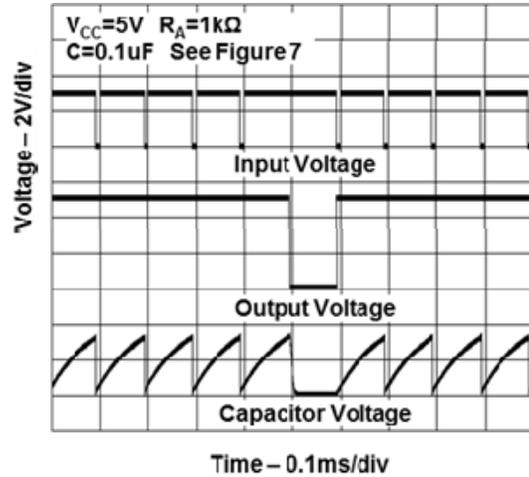
**Fig. 8 Timing Waveforms for Missing Pulse Detector**
