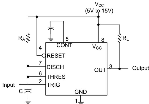
**Fig 1. Monostable operation**
