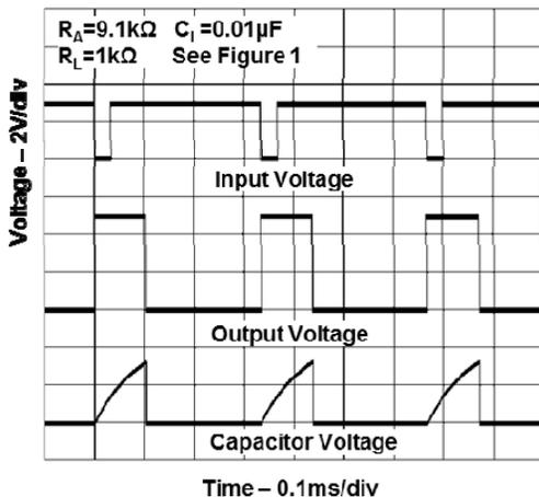
**Fig. 2 Typical Monostable Waveforms**
