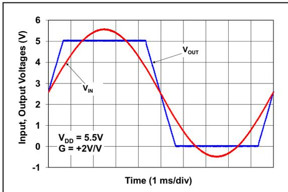
**FIGURE 2-33:** The MCP6421/2/4 Device Shows No Phase Reversal.
