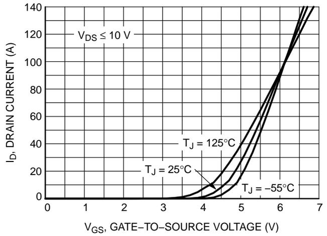
Figure 2. Transfer Characteristics
