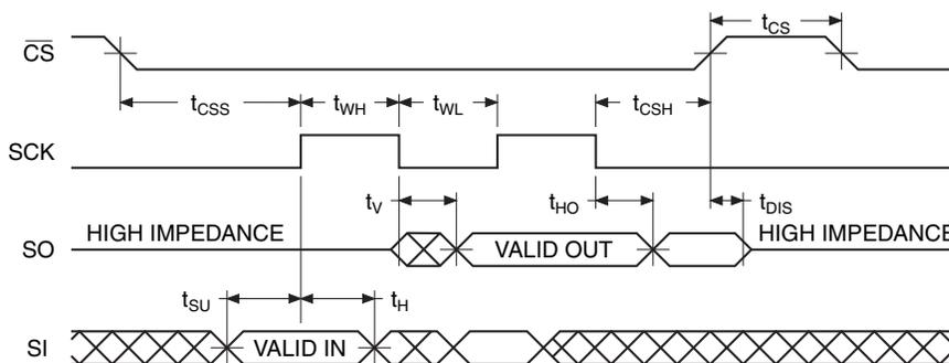
**21.2 Waveform 2 – SPI Mode 3 Compatible (for frequencies up to 66MHz)**
