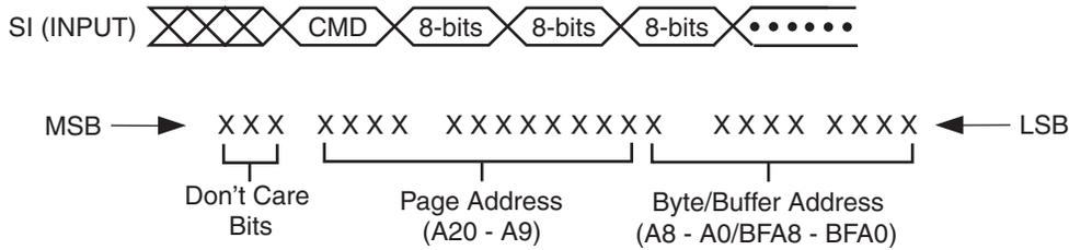
**21.8 Command Sequence for Read/Write Operations for Page Size 528-Bytes (Except Status Register Read, Manufacturer and Device ID Read)**
