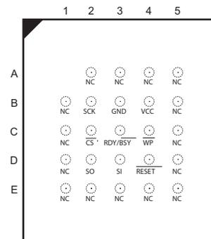
**Figure 2-3.** MLF (VDFN) Top View
