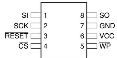
Note: 1. The metal pad on the bottom of the MLF package is floating. This pad can be a "No Connect" or connected to GND
