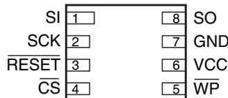
**Figure 2-4.** SOIC Top View
