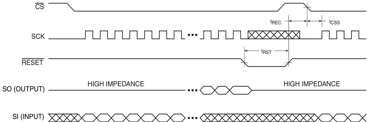
Note: The  $\overline{CS}$  signal should be in the high state before the  $\overline{RESET}$  signal is deasserted
