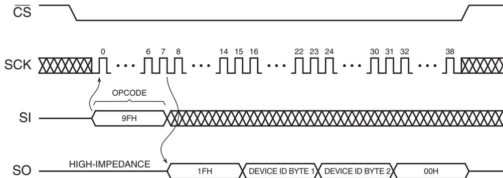
Note: Each transition
