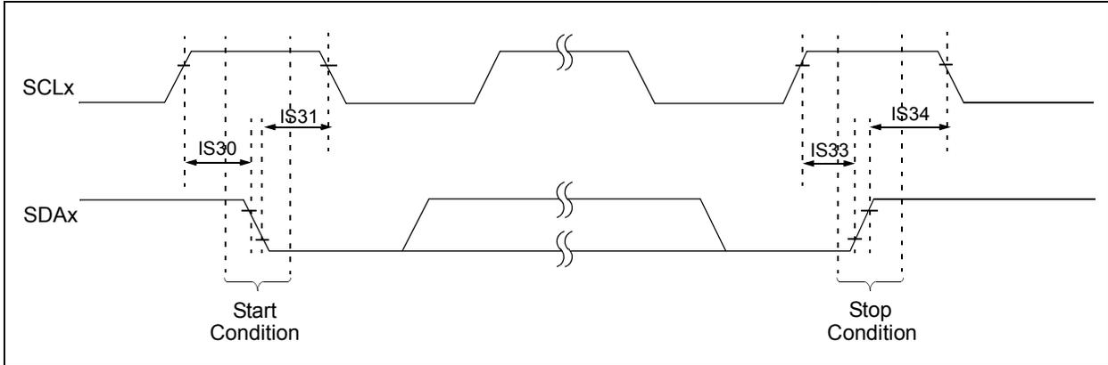
FIGURE 28-20: I2Cx BUS DATA TIMING CHARACTERISTICS (SLAVE MODE)
