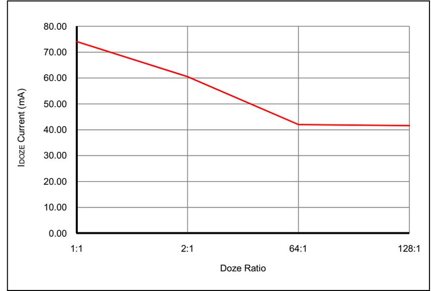
**FIGURE 32-10: TYPICAL I<sub>DD</sub> CURRENT @ V<sub>DD</sub> = 3.3V, +85°C**
