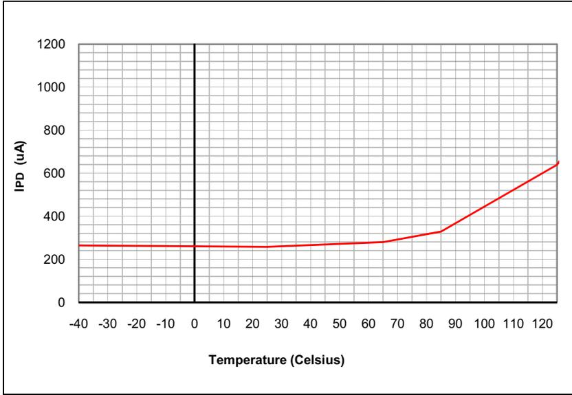
**FIGURE 32-11: TYPICAL I<sub>DOZE</sub> CURRENT @ V<sub>DD</sub> = 3.3V, +85°C**
