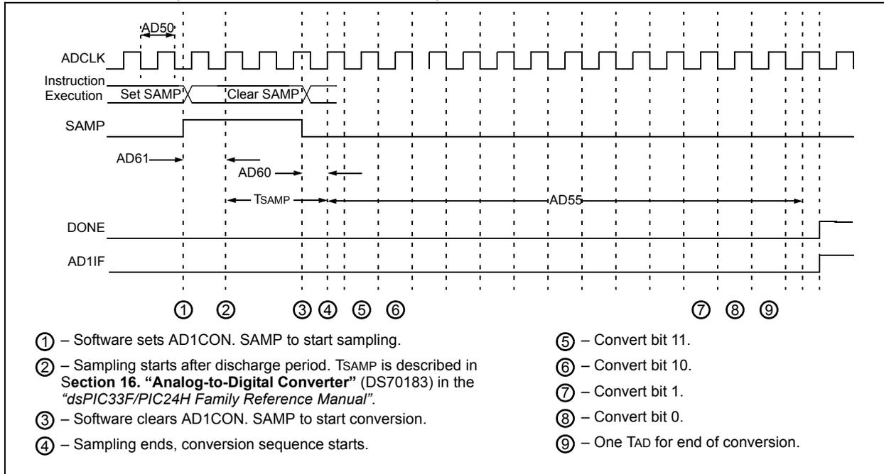
TABLE 28-42: ADC CONVERSION (12-BIT MODE) TIMING REQUIREMENTS
