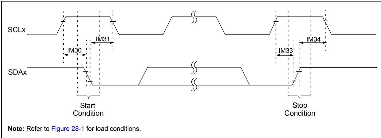
FIGURE 28-18: I2Cx BUS DATA TIMING CHARACTERISTICS (MASTER MODE)
