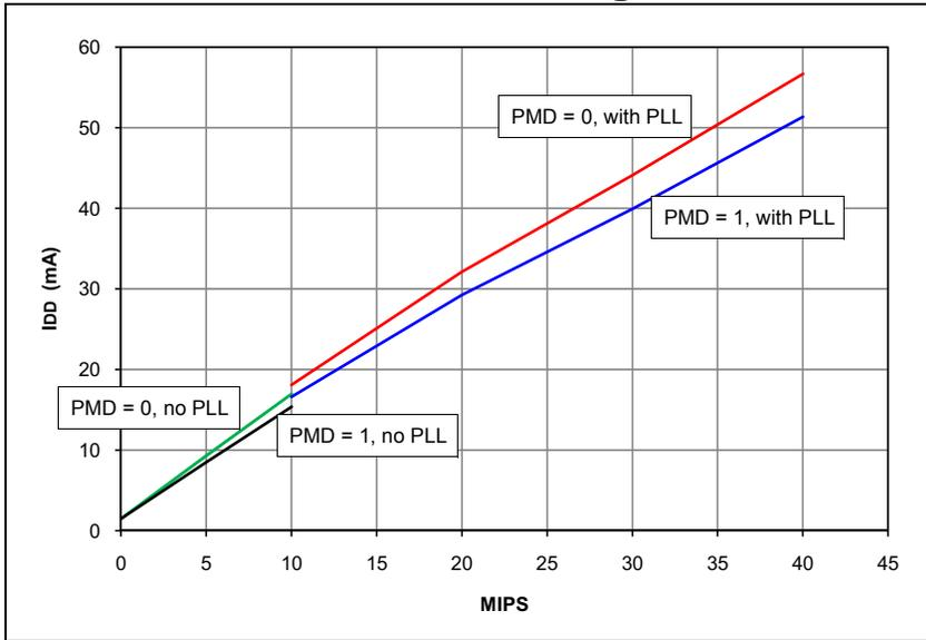
**FIGURE 32-12: TYPICAL I<sub>IDLE</sub> CURRENT @ V<sub>DD</sub> = 3.3V, +85°C**
