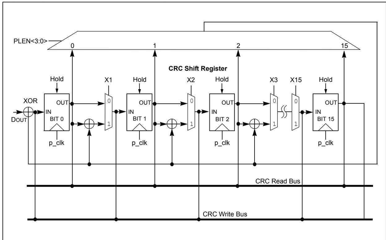
FIGURE 23-2: CRC GENERATOR RECONFIGURED FOR  $x^{16} + x^{12} + x^5 + 1$
