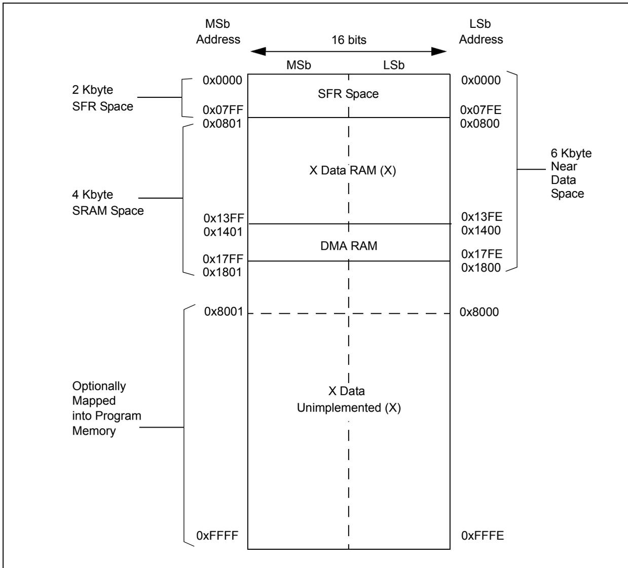
**FIGURE 4-4: DATA MEMORY MAP FOR PIC24HJ128GP202/204, PIC24HJ64GP202/204, PIC24HJ128GP502/504 AND PIC24HJ64GP502/504 DEVICES WITH 8 KB RAM**
