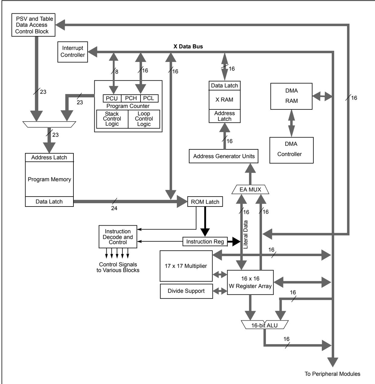
FIGURE 3-2: PIC24HJ32GP302/304, PIC24HJ64GPX02/X04 AND PIC24HJ128GPX02/X04 PROGRAMMER'S MODEL
