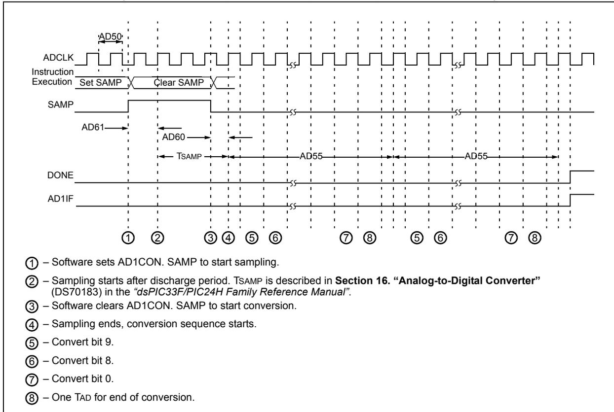
**FIGURE 28-24: ADC CONVERSION (10-BIT MODE) TIMING CHARACTERISTICS (CHPS<1:0> = 01, SIMSAM = 0, ASAM = 1, SSRC<2:0> = 111, SAMC<4:0> = 00001)**
