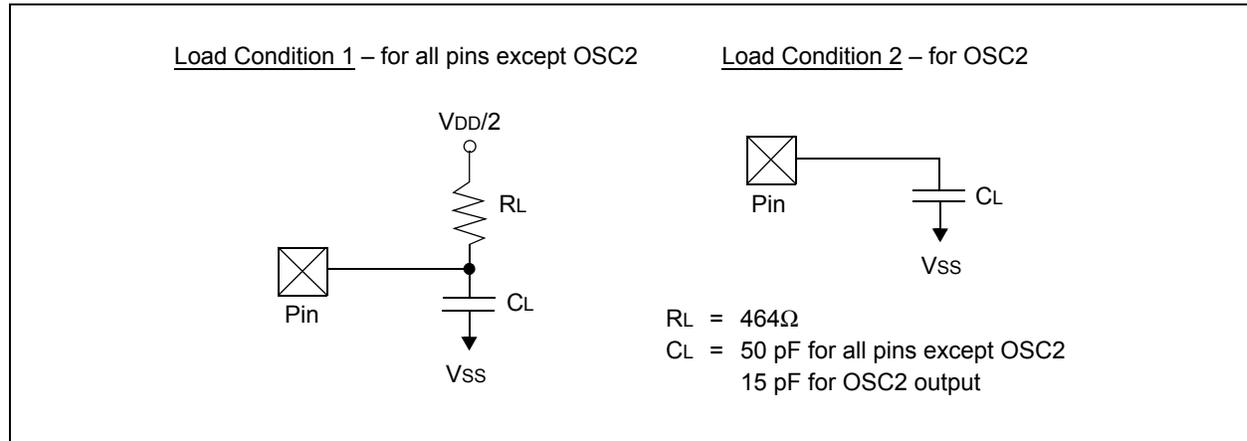
**TABLE 28-15: CAPACITIVE LOADING REQUIREMENTS ON OUTPUT PINS**
