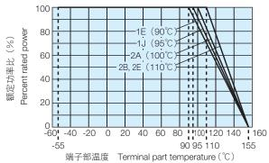
超过上述端子部温度使用时,请根据负荷减轻特性曲线减小额定功率后使用。 ※ 关于使用方法,请参照卷首的"端子部温度负荷减轻特性曲线的说明"。 For resistors operated terminal part temperature of described for each size or above, a power rating shall be derated in accordance with derating curve. \*Please refer to "Introduction of the derating curves based on the terminal part temperature" on the beginning of our catalog before use.
