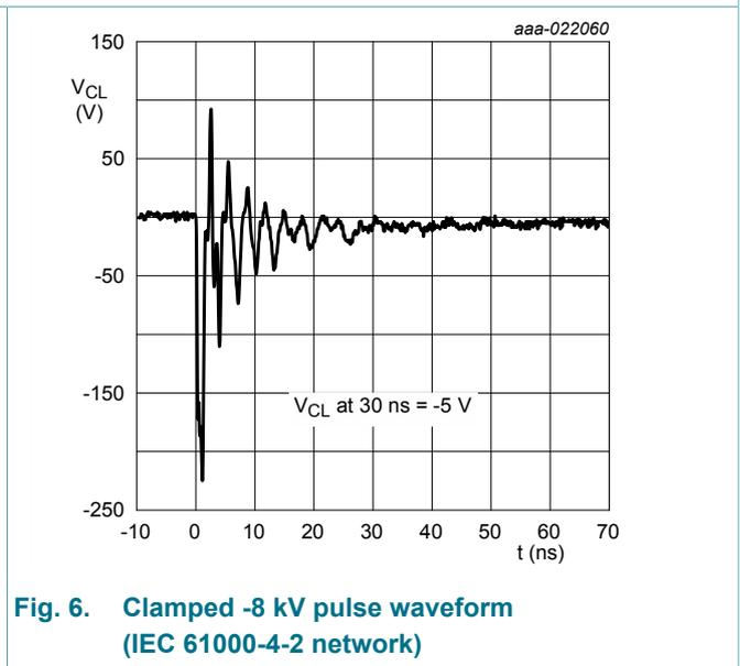
Fig. 6. Clamped -8 kV pulse waveform (IEC 61000-4-2 network)
