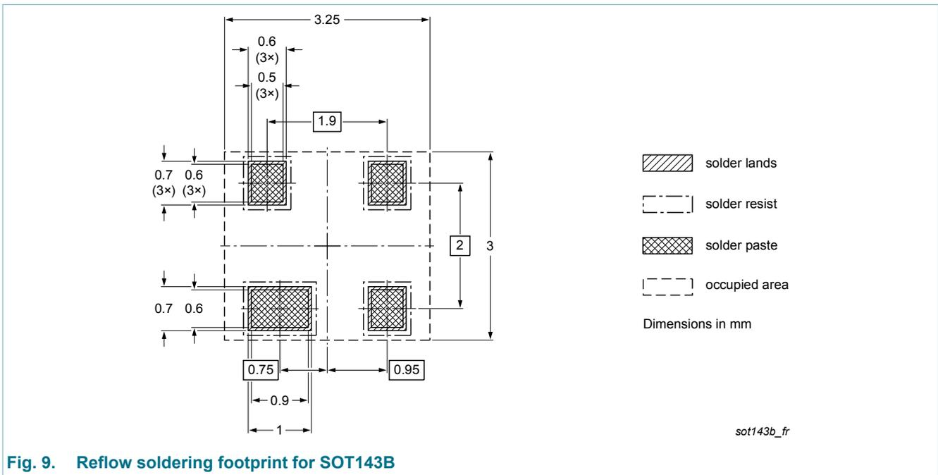
Fig. 9. Reflow soldering footprint for SOT143B
