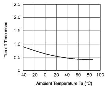
**Fig.5** LED operate vs. ambient temperature
