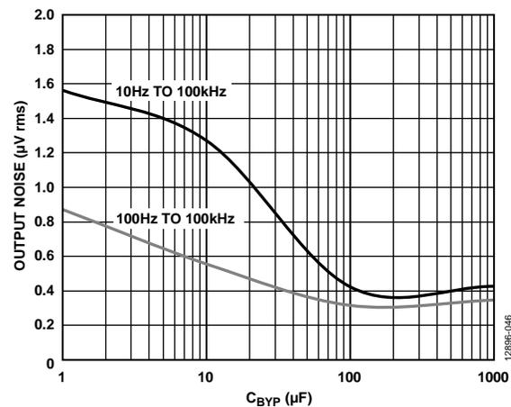
Figure 44. RMS Noise vs. Bypass Capacitance ( $C_{BYP}$ )
