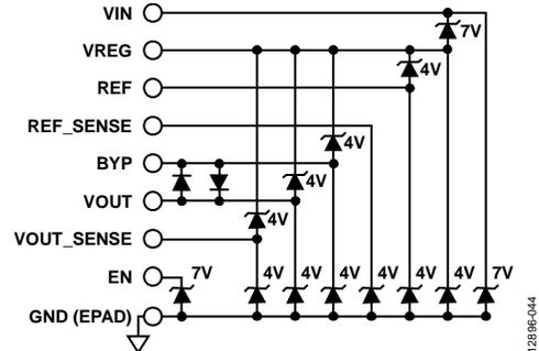
Figure 42. Simplified ESD Protection Block Diagram
