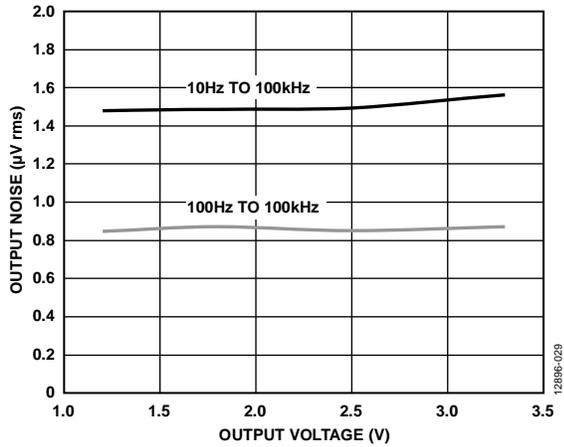
Figure 29. RMS Output Noise vs. Output Voltage
