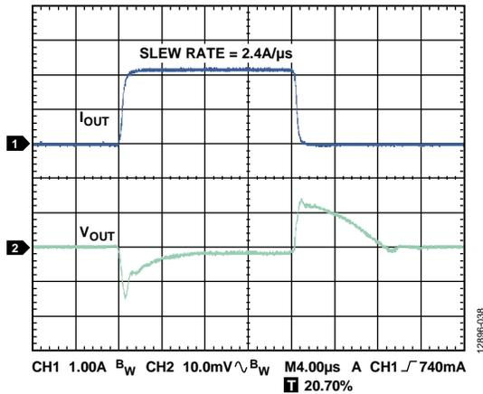
Figure 36. Load Transient Response,  $I_{LOAD} = 100 \text{ mA}$  to  $2 \text{ A}$ ,  $V_{OUT} = 1.8 \text{ V}$ ,  $V_{IN} = 2.5 \text{ V}$ ,  $C_{OUT} = 22 \mu\text{F}$ , Channel 1 =  $I_{OUT}$ , Channel 2 =  $V_{OUT}$
