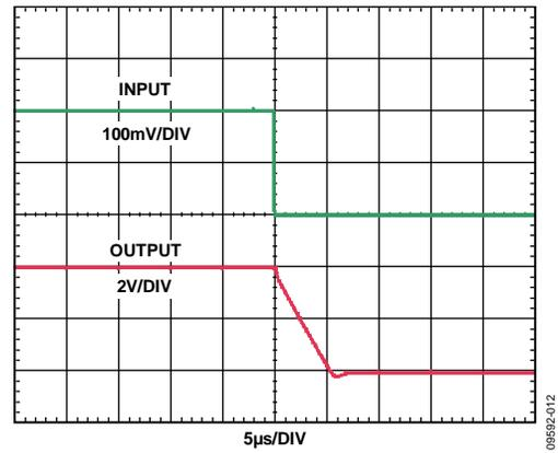
Figure 14. Fall Time (Differential Input = 200 mV)
