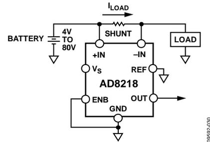
Figure 31. Enabling the Internal 80 mV Reference
