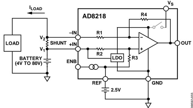
Figure 34. Bidirectional Operation Using a 2.5 V Reference Input
