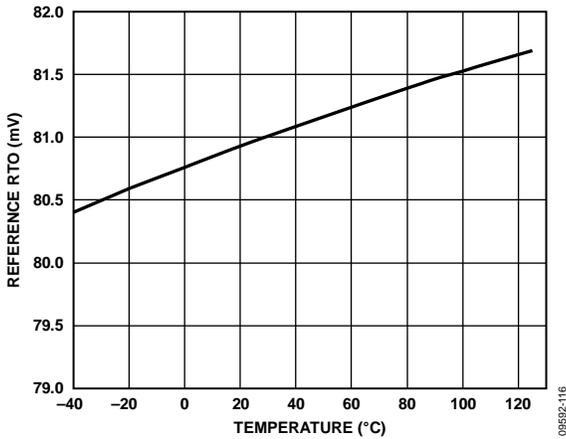
Figure 17. Internal Reference Voltage vs. Temperature
