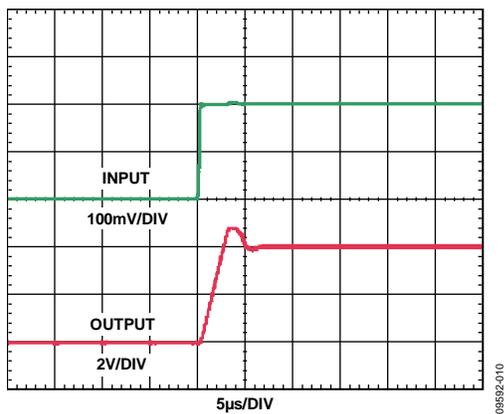
Figure 12. Rise Time (Differential Input = 200 mV)
