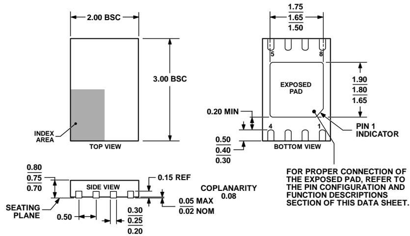
Figure 37. 8-Lead Lead Frame Chip Scale Package [LFCSP\_WD]
