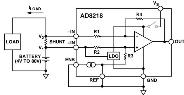
Figure 32. Unidirectional Operation with ENB Connected to GND
