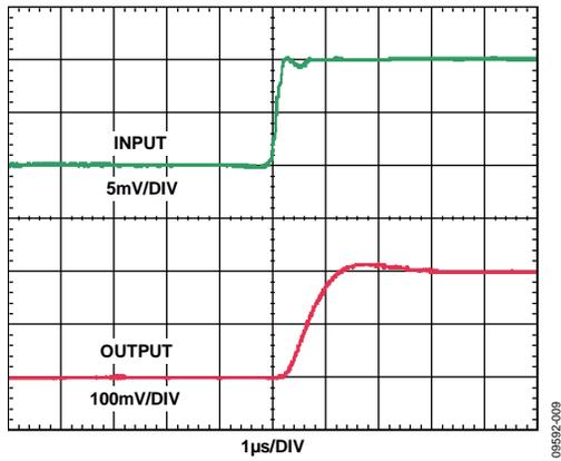
Figure 11. Rise Time (Differential Input = 10 mV)
