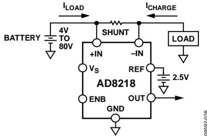
Figure 29. Operation with No V<sub>S</sub> Connection
