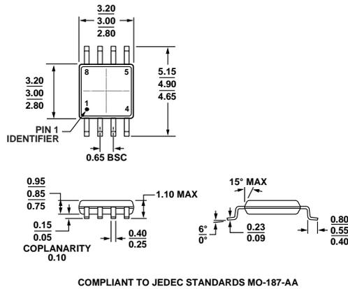
Figure 38. 8-Lead Mini Small Outline Package [MSOP]
