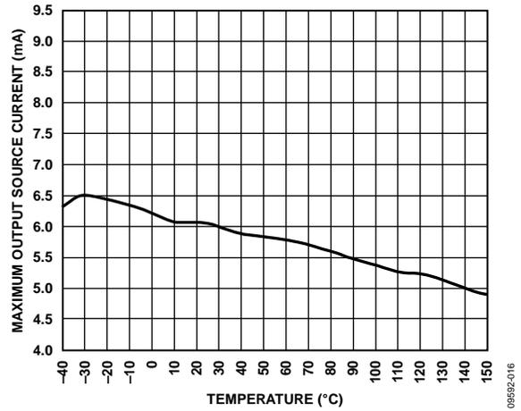
Figure 19. Maximum Output Source Current vs. Temperature
