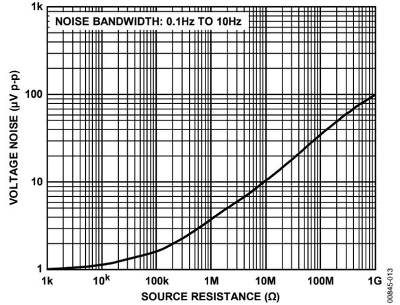
Figure 13. Input Voltage Noise vs. Source Resistance
