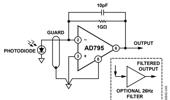
Figure 45. AD795 Used as a Photodiode Preamplifier
