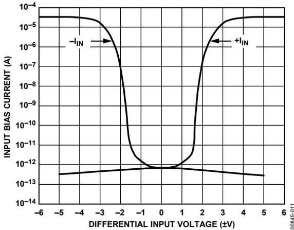
Figure 11. Input Bias Current vs. Differential Input Voltage
