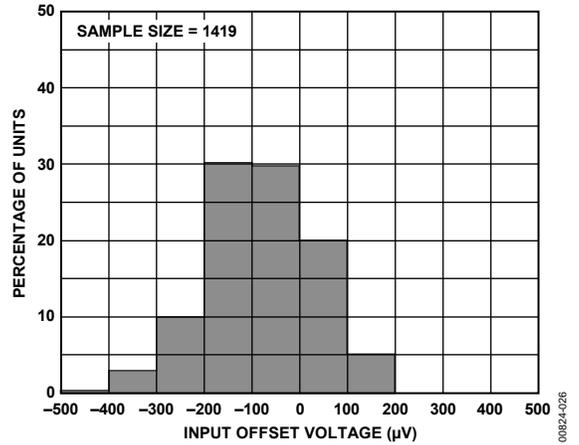
Figure 26. Typical Distribution of Input Offset Voltage
