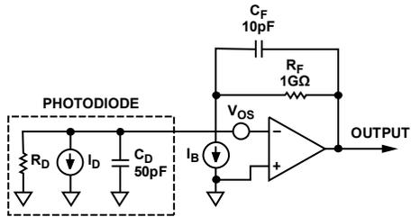
Figure 46. A Photodiode Model Showing DC Error Sources
