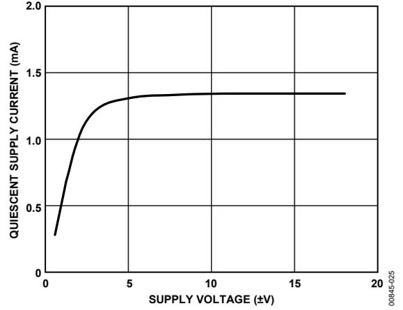
Figure 25. Quiescent Supply Current vs. Supply Voltage
