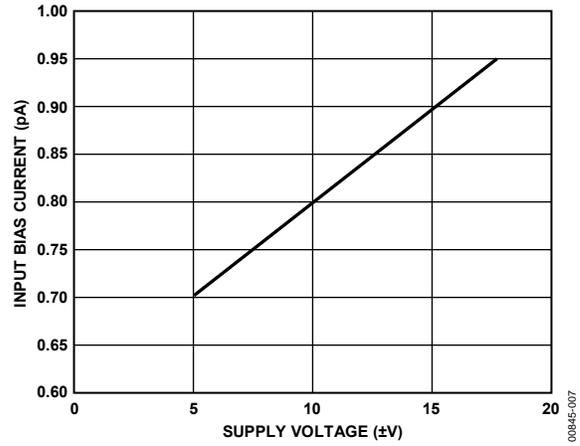
Figure 7. Input Bias Current vs. Supply Voltage
