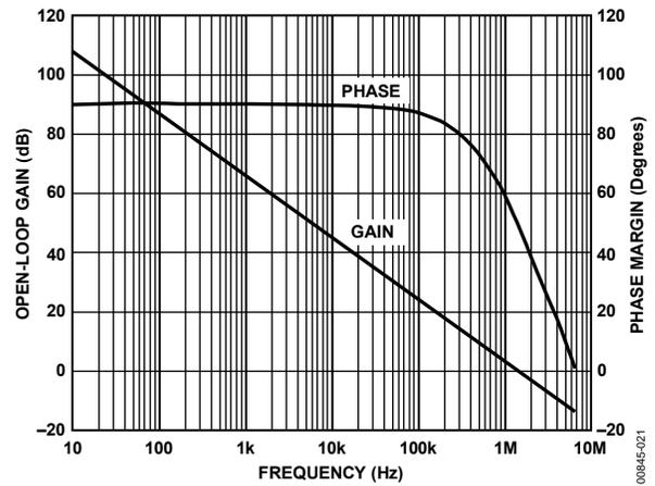
Figure 21. Open-Loop Gain and Phase Margin vs. Frequency
