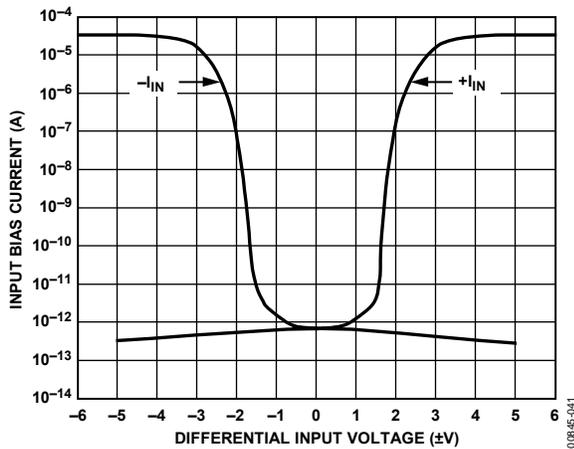
Figure 41. Input Bias Current vs. Differential Input Voltage
