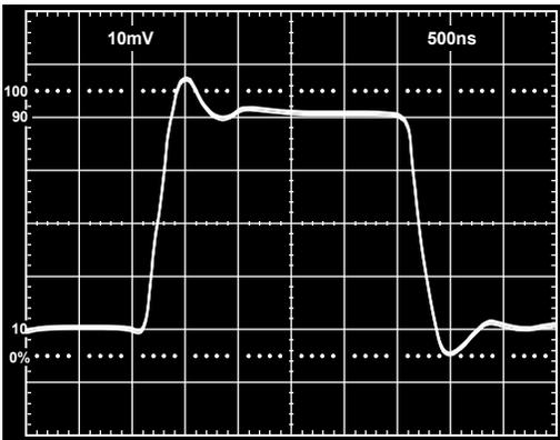
Figure 29. Unity Gain Inverter Small Signal Pulse Response
