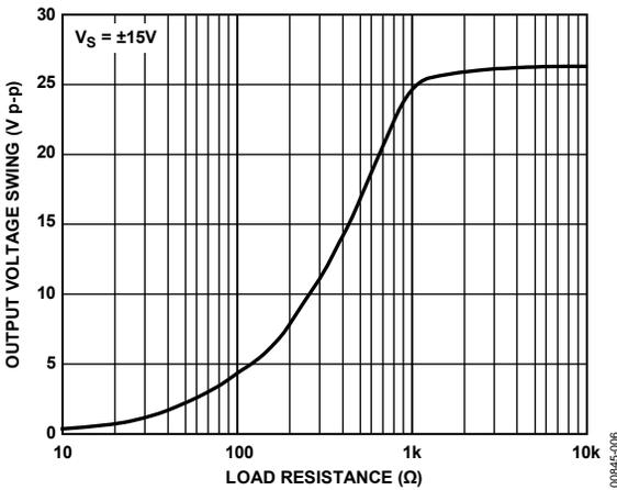
Figure 6. Output Voltage Swing vs. Load Resistance
