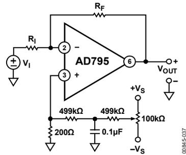
Figure 37. Alternate Offset Null Circuit for Inverter
