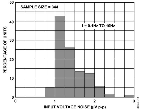
Figure 14. Typical Distribution of Input Voltage Noise
