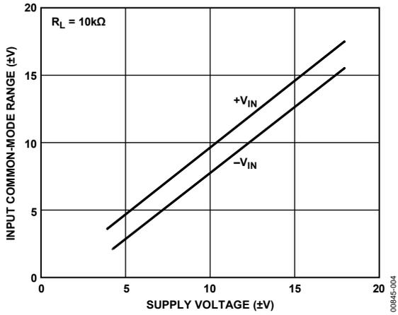
Figure 4. Common-Mode Voltage Range vs. Supply Voltage
