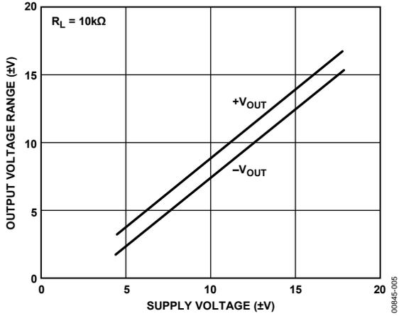
Figure 5. Output Voltage Range vs. Supply Voltage
