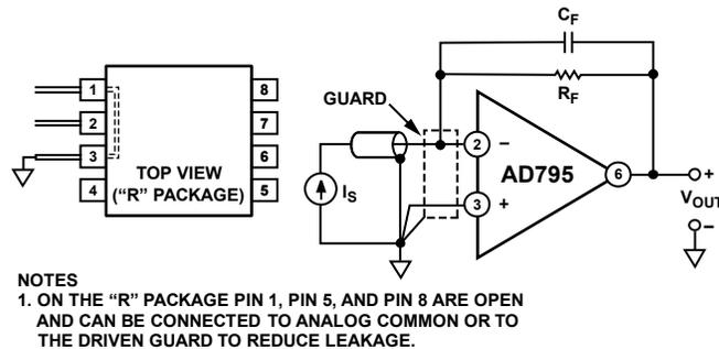
Figure 34. Guarding Scheme—Inverter
