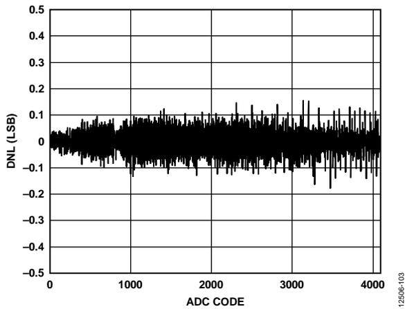
Figure 11. ADC DNL,  $V_{DD} = 5.5\text{ V}$
