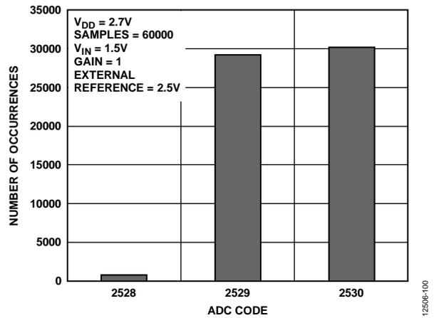
Figure 14. Histogram of ADC Codes,  $V_{DD} = 2.7\text{ V}$
