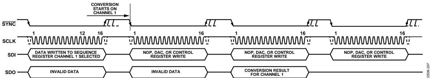
Figure 42. Single-Channel ADC Conversion Sequence, No Repeat
