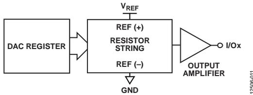
Figure 37. Internal Block Diagram of the DAC Architecture
