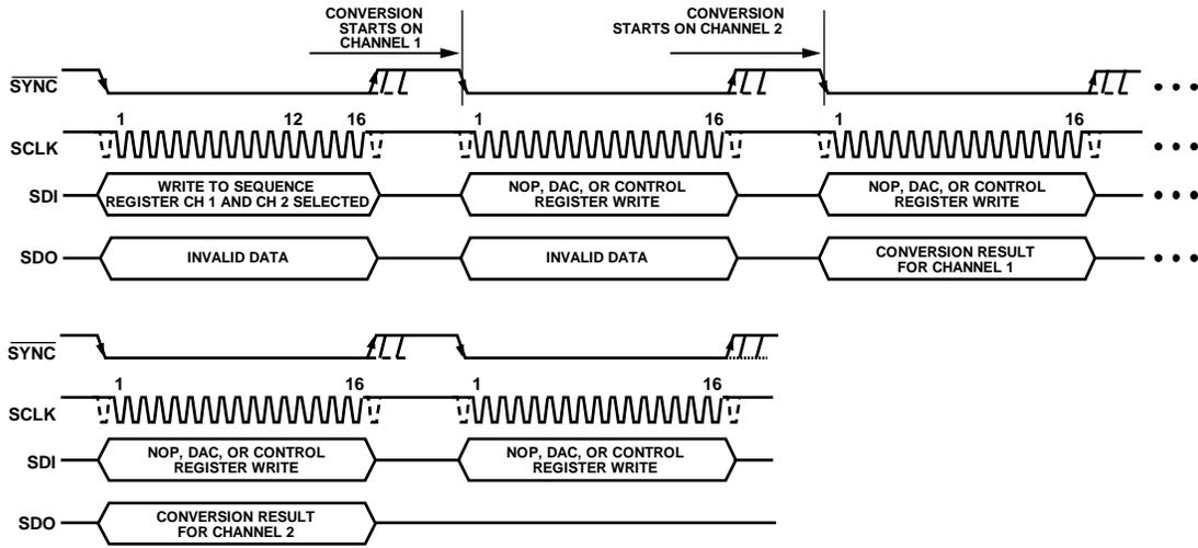
Figure 44. Multichannel ADC Conversion Sequence, No Repeat
