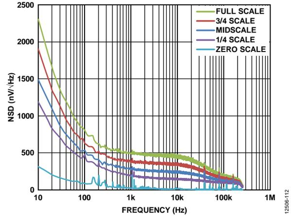
Figure 31. DAC Output Noise Spectral Density (NSD)
