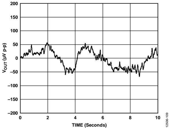
Figure 29. DAC 1/f Noise with External Reference
