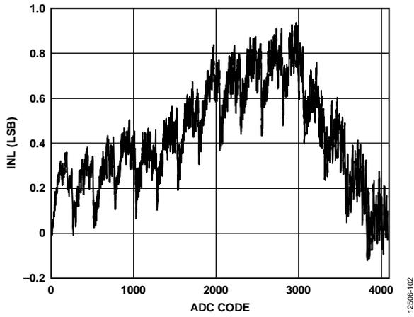
Figure 10. ADC INL,  $V_{DD} = 5.5\text{ V}$
