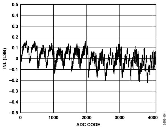
Figure 12. ADC INL,  $V_{DD} = 2.7\text{ V}$
