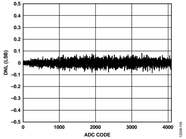
Figure 13. ADC DNL,  $V_{DD} = 2.7\text{ V}$
