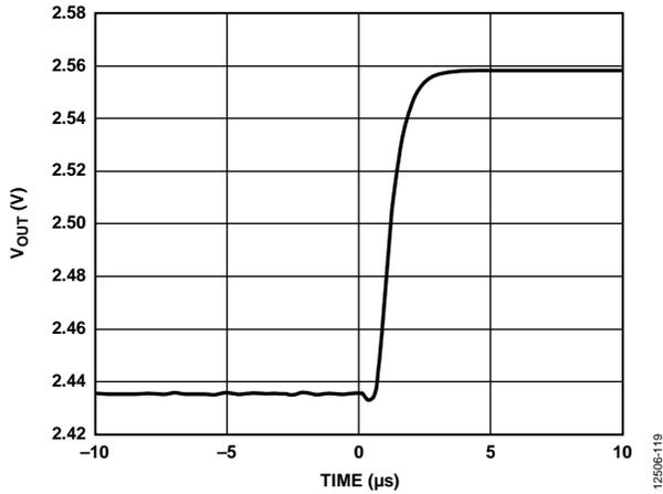
Figure 22. DAC Settling Time (100 Code Change, Rising Edge)
