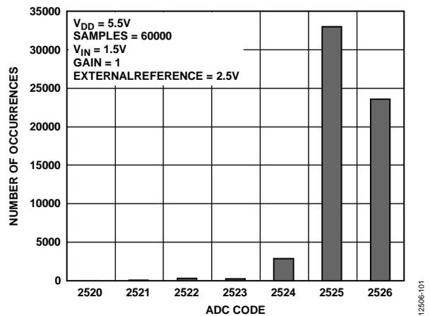
Figure 15. Histogram of ADC Codes,  $V_{DD} = 5.5\text{ V}$
