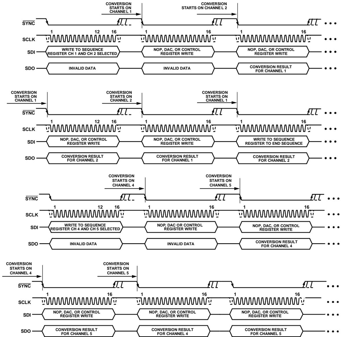
Figure 46. Changing a Multichannel, Repeating, ADC Conversion Sequence
