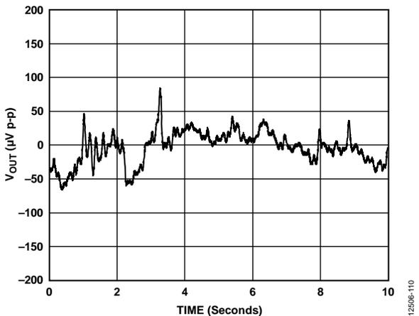
Figure 30. DAC 1/f Noise with Internal Reference
