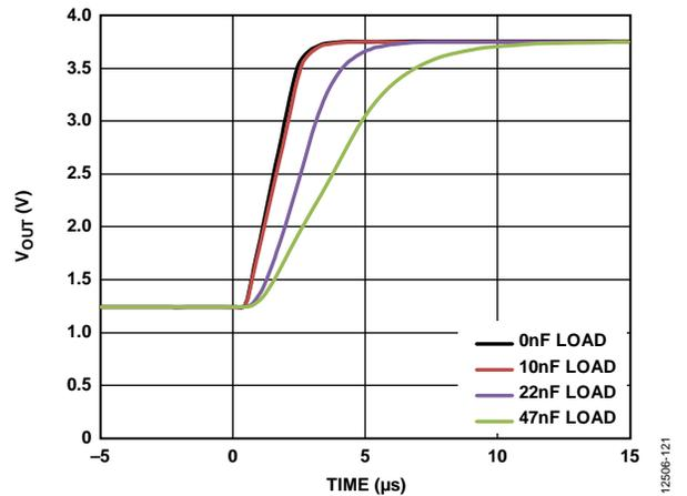
Figure 26. DAC Settling Time for Various Capacitive Loads
