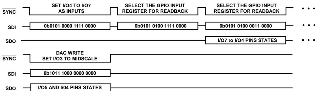
Figure 47. Configuring and Reading General-Purpose Input Pins
