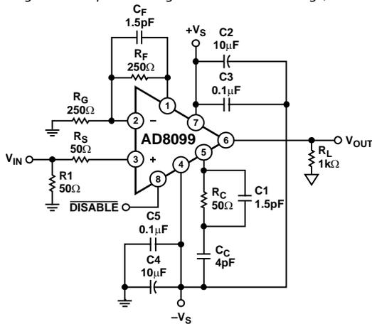
Figure 61. Amplifier Configuration for SOIC Package, Gain = +2
