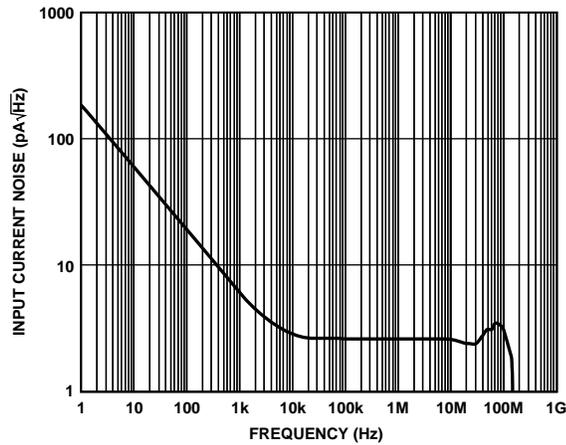
Figure 48. Input Current Noise vs. Frequency ( $\overline{DISABLE} = Open$ )
