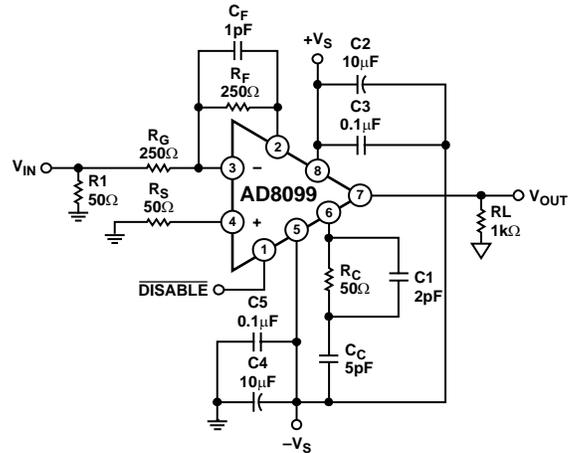
Figure 62. Amplifier Configuration for LFCSP, Gain = -1
