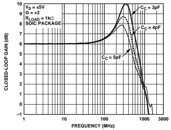
Figure 73. Frequency Response for Various Values of  $C_C$
