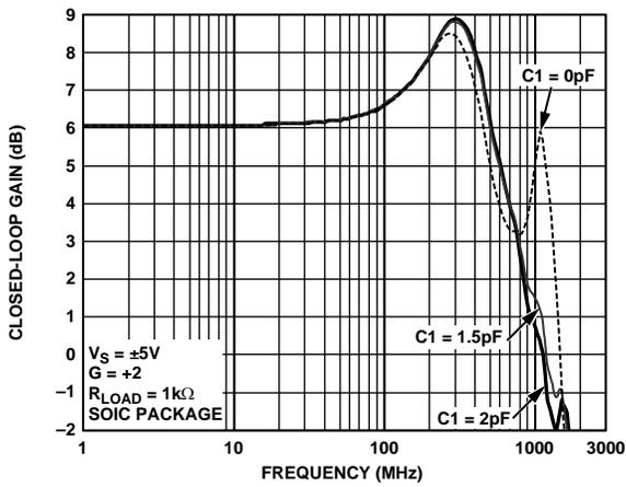
Figure 72. Frequency Response for Various Values of  $C_1$
