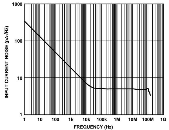
Figure 51. Input Current Noise vs. Frequency ( $\overline{DISABLE} = +Vs$ )
