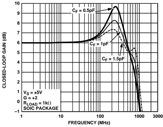
Figure 71. Frequency Response for Various Values of  $C_F$
