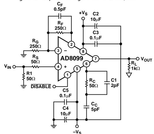
Figure 63. Amplifier Configuration for LFCSP, Gain = +2
