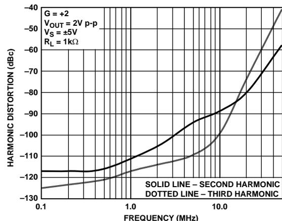
Figure 3. Harmonic Distortion vs. Frequency and Gain (SOIC)
