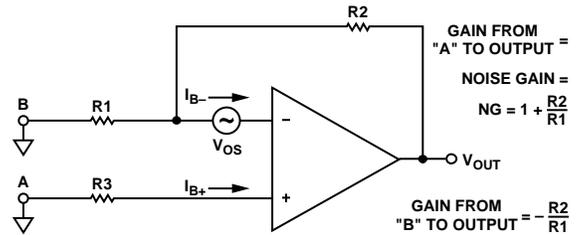
◆ OFFSET (RTO) =  $V_{OS} \left[ 1 + \frac{R2}{R1} \right] + I_{B+} \times R3 \left[ 1 + \frac{R2}{R1} \right] - I_{B-} \times R2$
