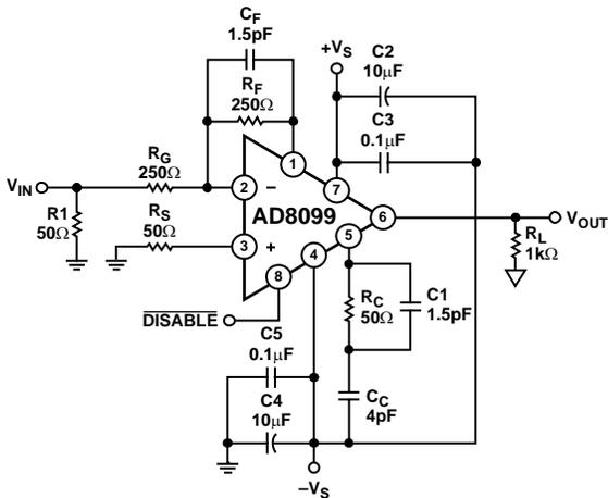
Figure 60. Amplifier Configuration for SOIC Package, Gain = -1
