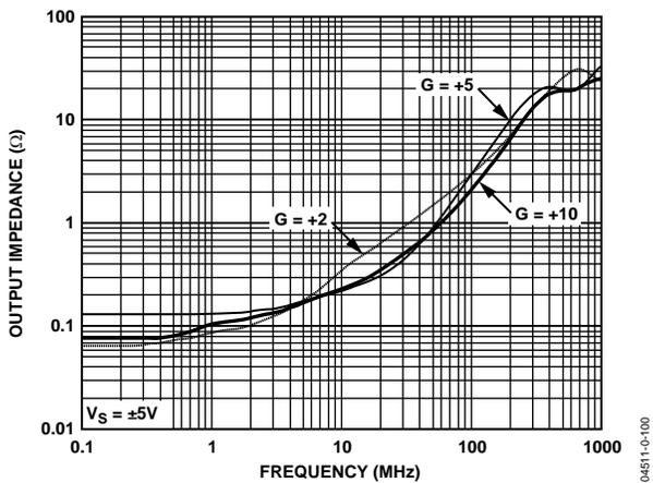
Figure 19. Output Impedance vs. Frequency for Various Gains
