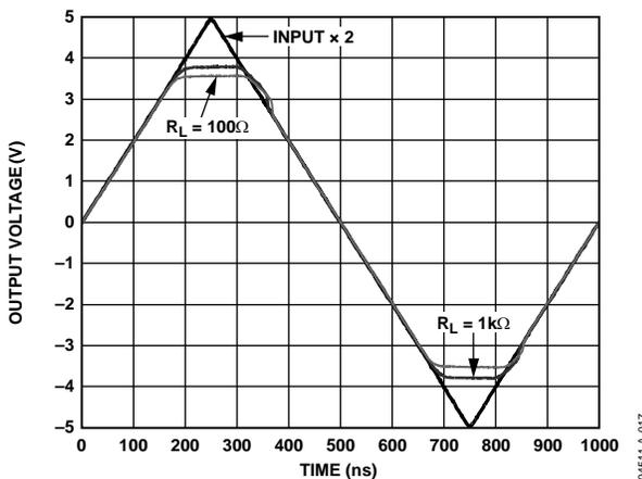
Figure 37. Output Overdrive Recovery for Various Resistive Loads
