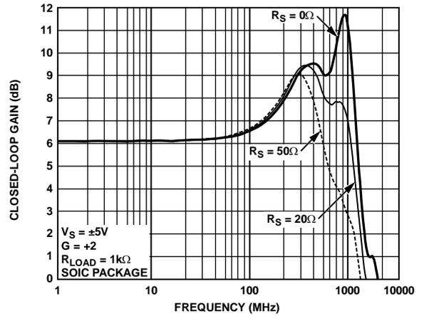
Figure 69. Frequency Response for Various Values of  $R_S$
