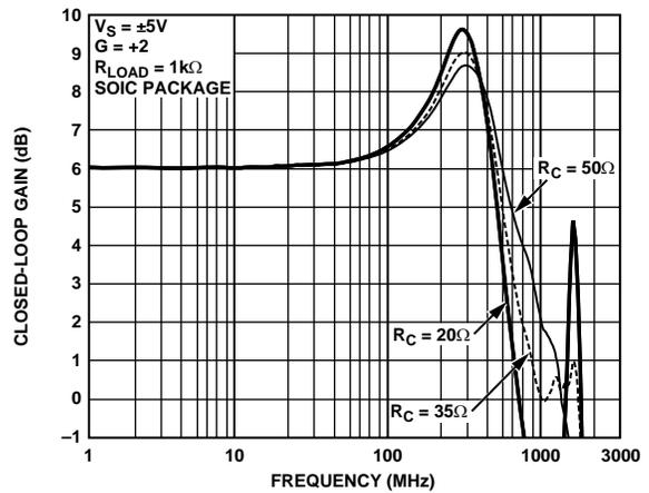
Figure 70. Frequency Response for Various Values of  $R_C$
