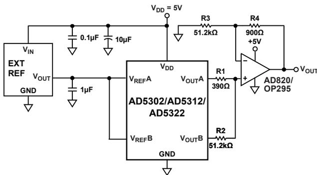
Figure 44. Coarse/Fine Adjustment
