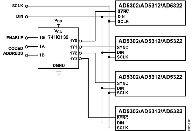
Figure 42. Decoding Multiple AD5302/AD5312/AD5322 Devices in a System
