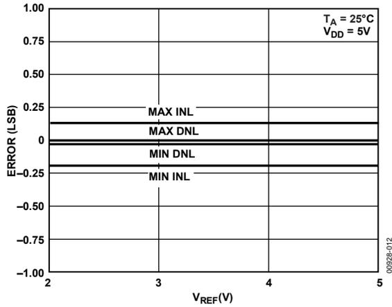
Figure 12. AD5302 INL and DNL Error vs.  $V_{REF}$
