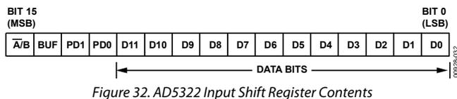
The remaining bits are DAC data bits, starting with the MSB and ending with the LSB. The AD5322 uses all 12 bits of DAC data, the AD5312 uses 10 bits and ignores the 2 LSB. The AD5302 uses eight bits and ignores the last four bits. The data format is straight binary, with all 0s corresponding to 0 V output, and all 1s corresponding to full-scale output ( $V_{REF} - 1 \text{ LSB}$ ).
