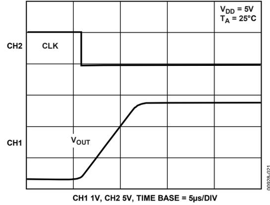
Figure 21. Half-Scale Setting ( $1/4$  to  $3/4$  Scale Code Change)
