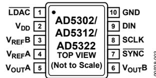
Figure 5. Pin Configuration
