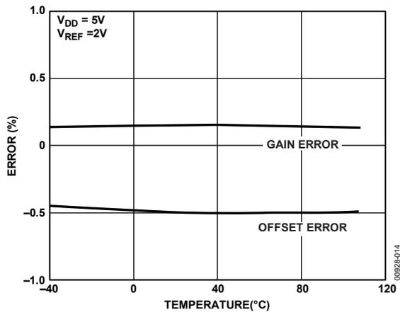
Figure 14. Offset Error and Gain Error vs. Temperature
