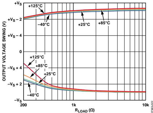
Figure 23. Output Voltage Swing vs.  $R_{LOAD}$
