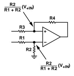
Figure 44. Voltage Division in the Difference Amplifier Configuration
