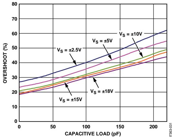
Figure 29. Small-Signal Overshoot vs. Capacitive Load, Gain = 1
