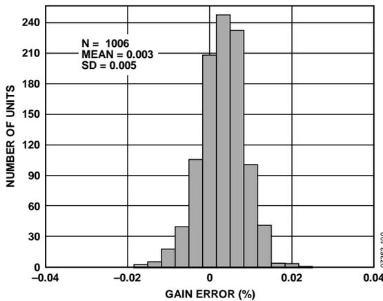
Figure 6. Typical Distribution of Gain Error, Gain = 1
