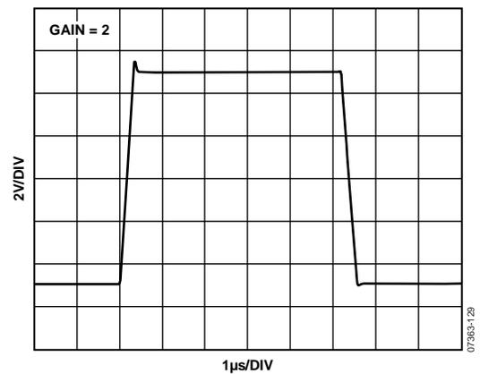
Figure 33. Large-Signal Pulse Response, Gain = 2
