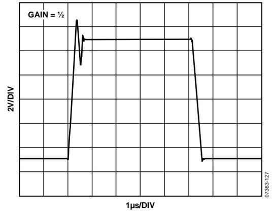
Figure 31. Large-Signal Pulse Response, Gain =  $\frac{1}{2}$
