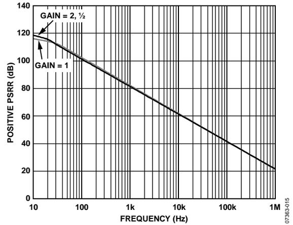
Figure 19. Positive PSRR vs. Frequency
