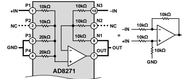
Figure 46. Gain = 1 Difference Amplifier, Referenced to Ground
