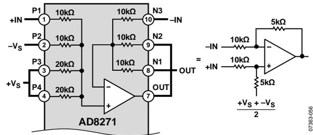
Figure 48. Gain =  $\frac{1}{2}$  Difference Amplifier, Referenced to Midsupply
