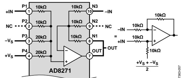
Figure 49. Gain = 1 Difference Amplifier, Referenced to Midsupply
