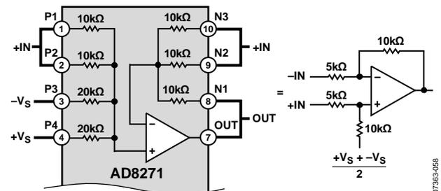
Figure 50. Gain = 2 Difference Amplifier, Referenced to Midsupply
