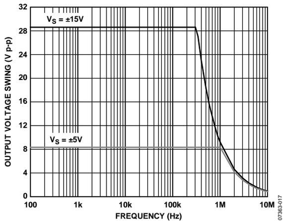
Figure 18. Output Voltage Swing vs. Large-Signal Frequency Response
