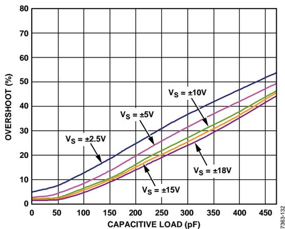
Figure 30. Small-Signal Overshoot vs. Capacitive Load, Gain = 2
