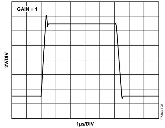
Figure 32. Large-Signal Pulse Response, Gain = 1
