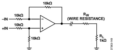
Figure 51. Wire Resistance Causes Errors at Load Voltage
