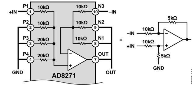
Figure 45. Gain =  $\frac{1}{2}$  Difference Amplifier, Referenced to Ground
