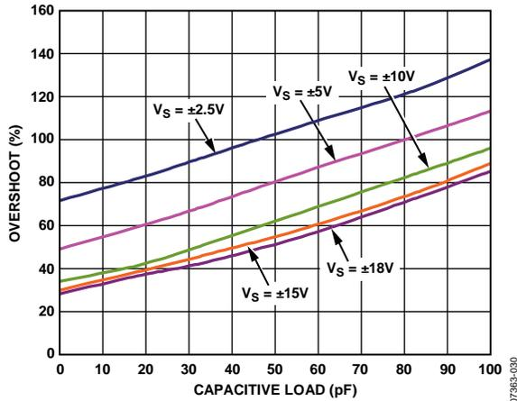
Figure 28. Small-Signal Overshoot vs. Capacitive Load, Gain =  $\frac{1}{2}$
