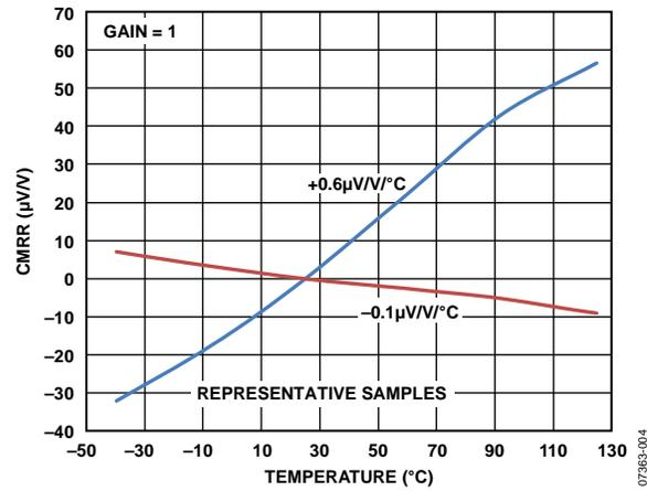
Figure 7. CMRR vs. Temperature, Normalized at  $25^\circ\text{C}$ , Gain = 1
