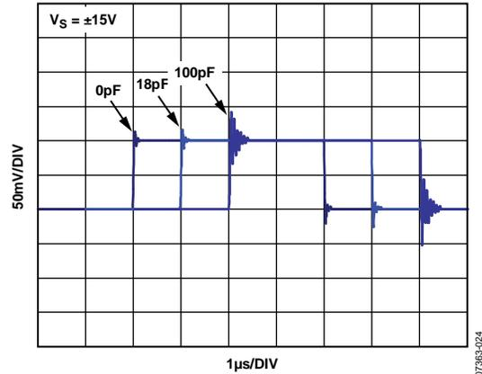
Figure 25. Small-Signal Step Response, Gain = 1/2
