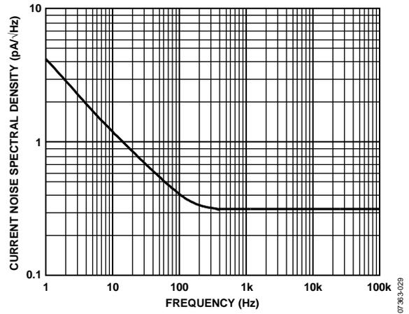
Figure 42. Current Noise Spectral Density vs. Frequency
