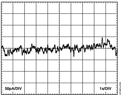
Figure 41. 0.1 Hz to 10 Hz Current Noise
