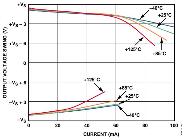
Figure 24. Output Voltage Swing vs. Current ( $I_{OUT}$ )
