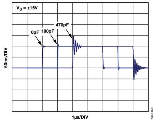
Figure 27. Small-Signal Step Response, Gain = 2
