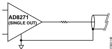
Figure 55. Driving Cabling
