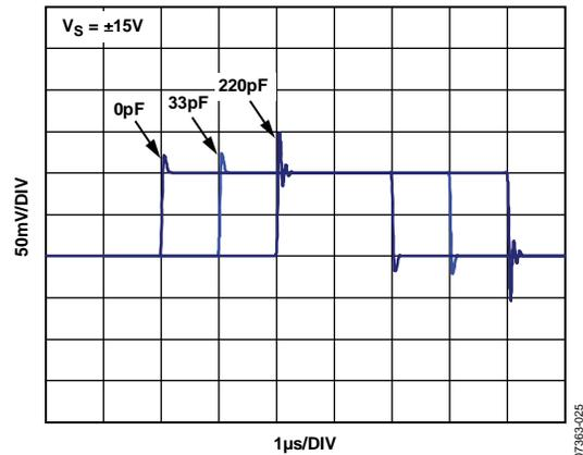
Figure 26. Small-Signal Step Response, Gain = 1
