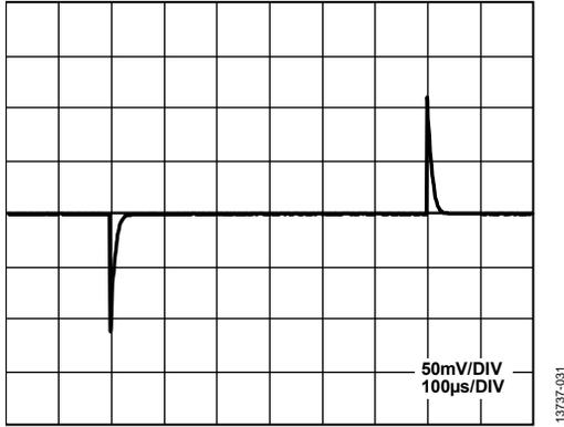
Figure 31. Load Transient Response (100 µA Load Change)
