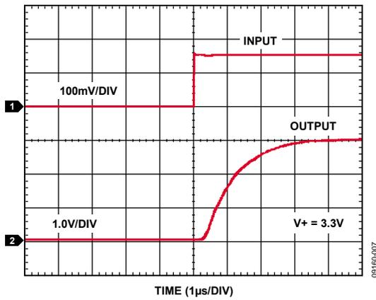
Figure 10. Rise Time ( $V^+ = 3.3\text{ V}$ )
