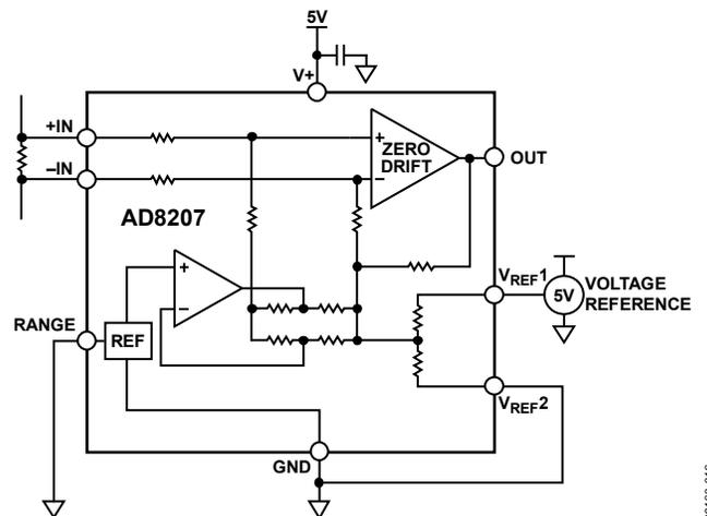
Figure 32. Splitting an External Reference,  $V_+ = 5\text{ V}$
