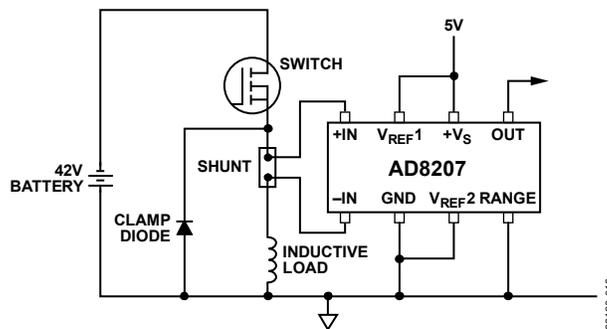
Figure 36. High-Side Switch
