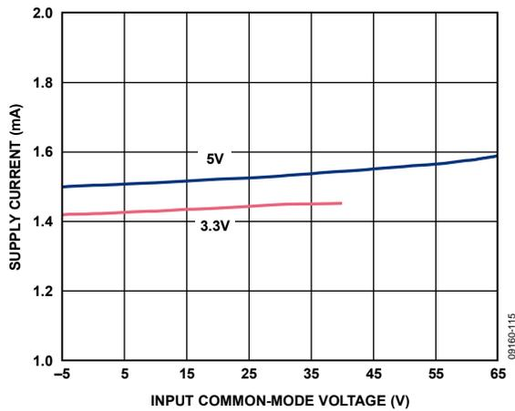
Figure 9. Supply Current vs. Input Common-Mode Voltage
