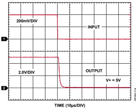
Figure 17. Differential Overload Recovery, Falling ( $V+ = 5V$ )
