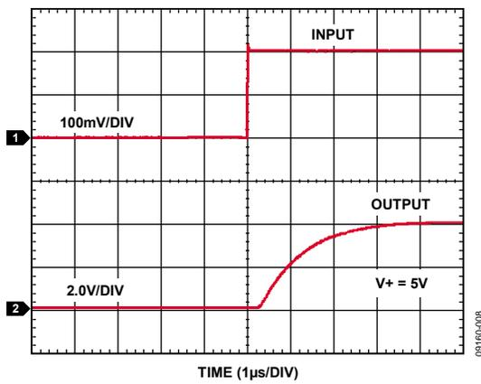
Figure 11. Rise Time ( $V^+ = 5\text{ V}$ )
