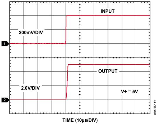
Figure 15. Differential Overload Recovery, Rising ( $V+ = 5V$ )
