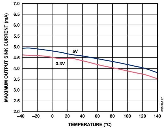
Figure 19. Maximum Output Sink Current vs. Temperature
