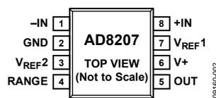
Figure 2. Pin Configuration
