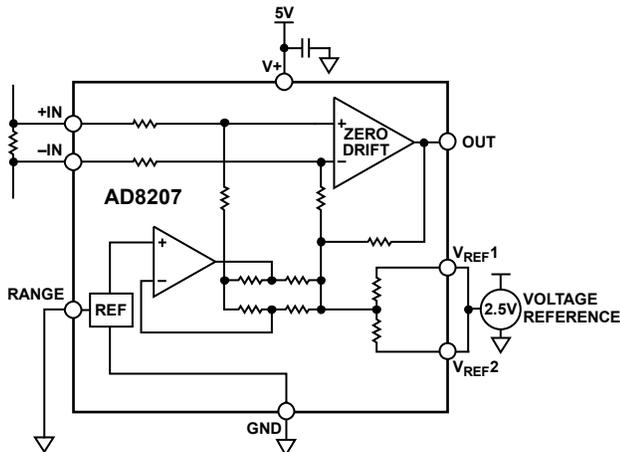
Figure 30. External Referenced Output,  $V_+ = 5\text{ V}$
