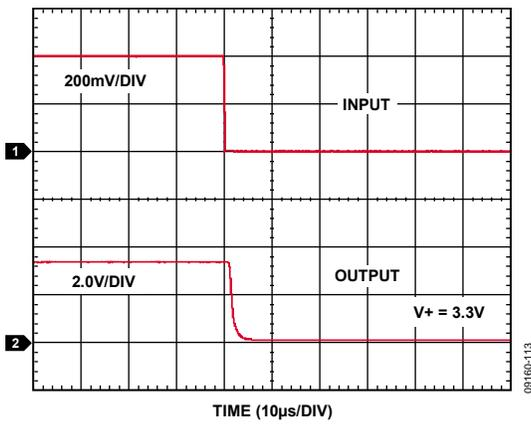
Figure 16. Differential Overload Recovery, Falling ( $V+ = 3.3V$ )
