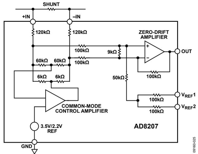
Figure 25. Simplified Schematic
