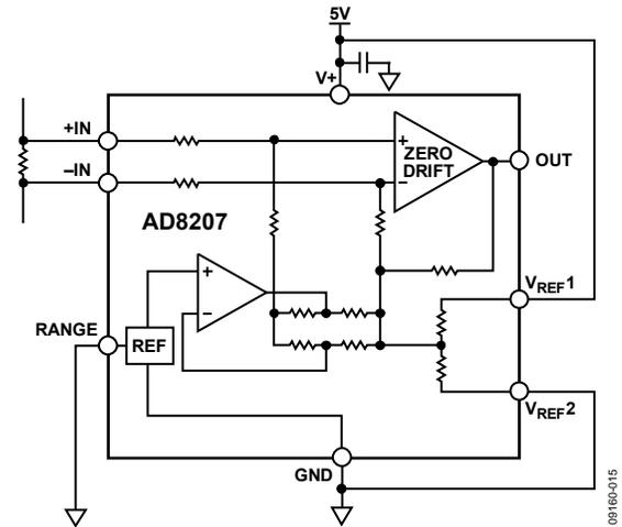
Figure 31. Splitting the Supply,  $V_+ = 5\text{ V}$
