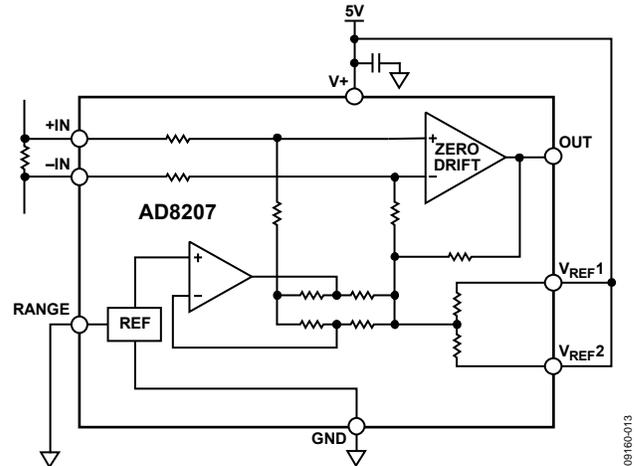
Figure 29. V+ Referenced Output Mode, V+ = 5 V
