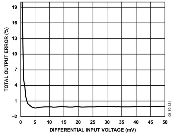
Figure 7. Total Output Error vs. Differential Input Voltage
