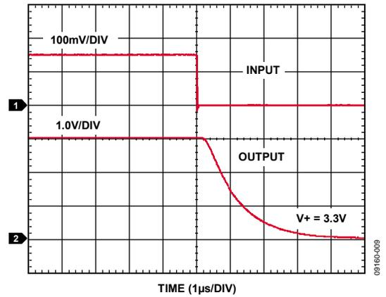
Figure 12. Fall Time ( $V^+ = 3.3\text{ V}$ )
