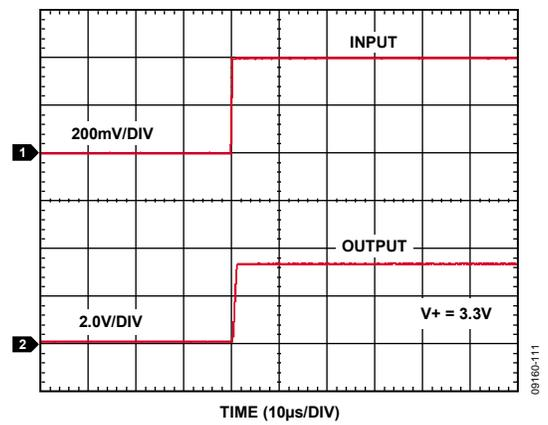
Figure 14. Differential Overload Recovery, Rising ( $V^+ = 3.3\text{ V}$ )
