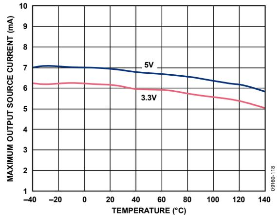
Figure 20. Maximum Output Source Current vs. Temperature
