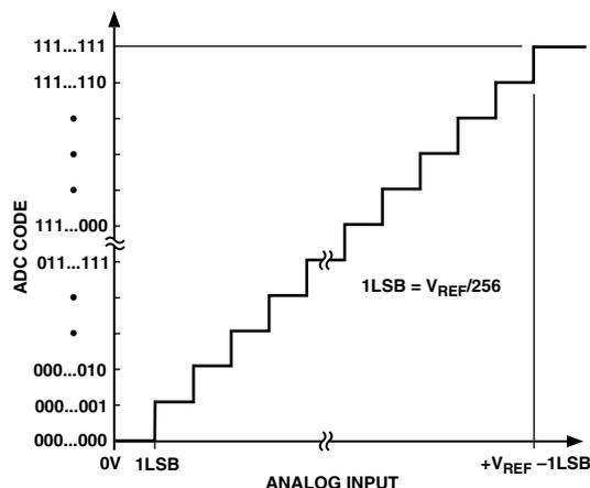
Figure 11. Transfer Characteristic
