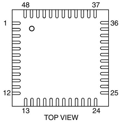
Figure 4-6. Orientation of the 48-lead LQFP Package
