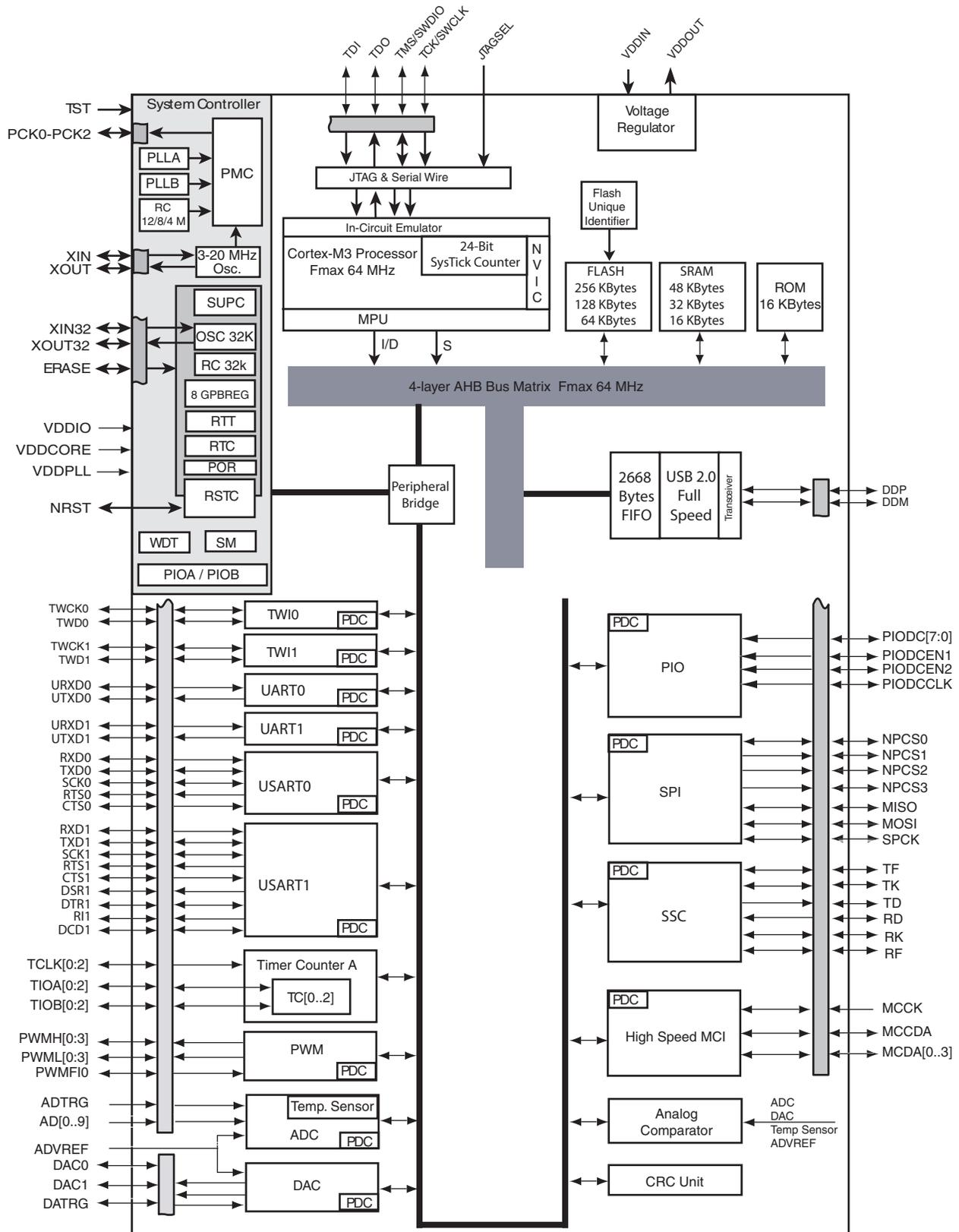
Figure 2-3. SAM3S 48-pin Version Block Diagram
