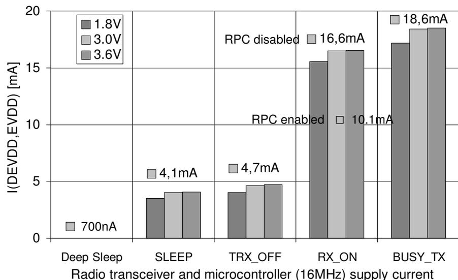
The transmit output power is set to maximum. If the radio transceiver is in SLEEP mode the current is dissipated by the AVR microcontroller only.
