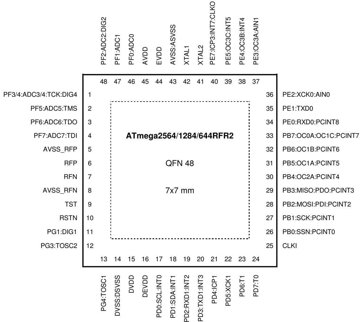
Note: The large center pad underneath the QFN/MLF package is made of metal and internally connected to AVSS. It should be soldered or glued to the board to ensure good mechanical stability. If the center pad is left unconnected, the package might loosen from the board. It is not recommended to use the exposed paddle as a replacement of the regular AVSS pins.
