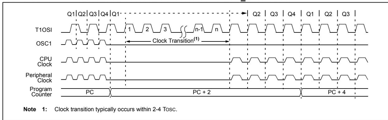
**FIGURE 3-2: TRANSITION TIMING FROM SEC\_RUN MODE TO PRI\_RUN MODE (HSPLL)**
