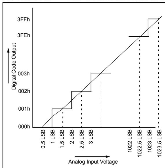
**FIGURE 21-3: ANALOG INPUT MODEL**
