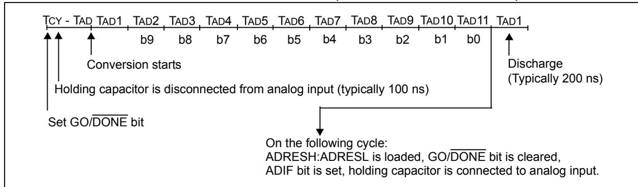
**FIGURE 21-5: A/D CONVERSION TAD CYCLES (ACQT<2:0> = 010, TACQ = 4 TAD)**
