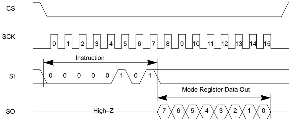
**Figure 9. SPI Read Mode Register Sequence (RDMR)**
