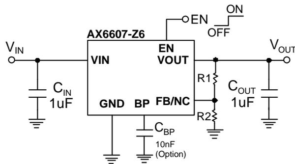
$$V_{OUT} = V_{FB} * (1 + R1/R2)$$
