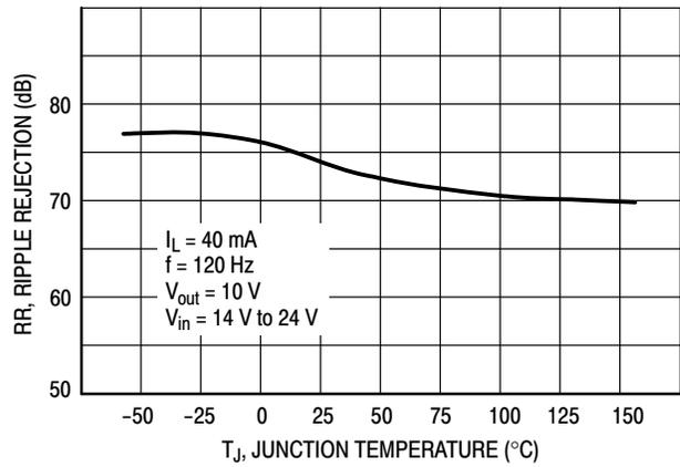
Figure 7. Ripple Rejection
