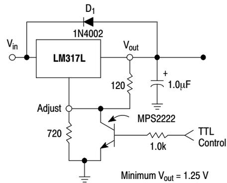
$D_1$  protects the device during an input short circuit.
