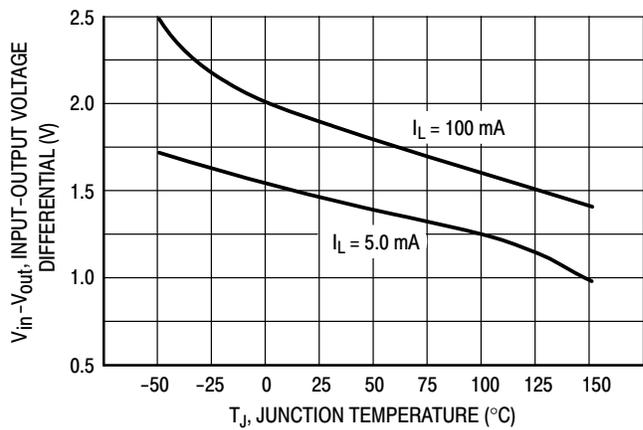
Figure 9. Dropout Voltage
