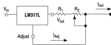
$$I_{outmax} = \left( \frac{V_{ref}}{R_1} \right) + I_{Adj} \cong \frac{1.25 \text{ V}}{R_1}$$
