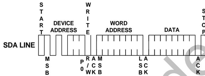
Figure 5: Byte Write
